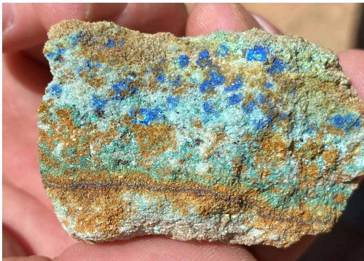
Figure 1: Coarsely disseminated copper oxides (in this case azurite – brilliant blue in colour) are widespread in outcrop throughout the Copper Warrior Project area.
