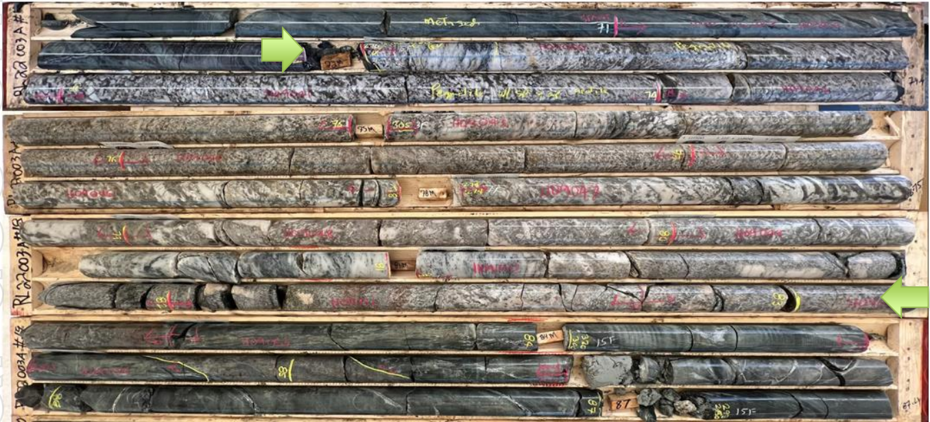
Figure 3: RL-22-003 – Whole NQ diamond core showing high density spodumene crystal laths, 11.5m @ 2.03% Li 2 O
