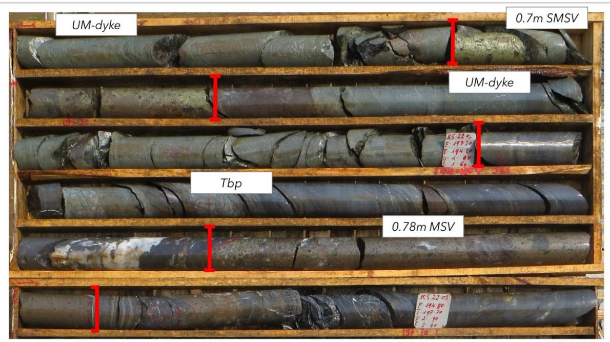
**Image 1** – King Snake hole KS22-05 massive Ni-Cu-Co-PGE sulfide veins associated with ultramafic dykes intruding Ban the Phuc horizon (Tbp), 6.2m @ 0.73% Ni, 0.89% Cu, 0.02% Co & 3.32g/t PGE from 191.8m, including **0.7m @ 1.1% Ni, 4.73% Cu, 0.05% Co & 18.2g/t PGE<sup>1</sup>** from 192.65m & **0.78m @ 2.36% Ni, 0.74% Cu, 0.09% Co & 2.09g/t PGE** from 196.35m
