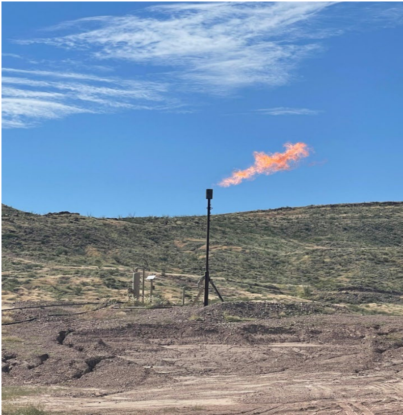
Above picture is of gas being flared during testing of Presidio 141#2
