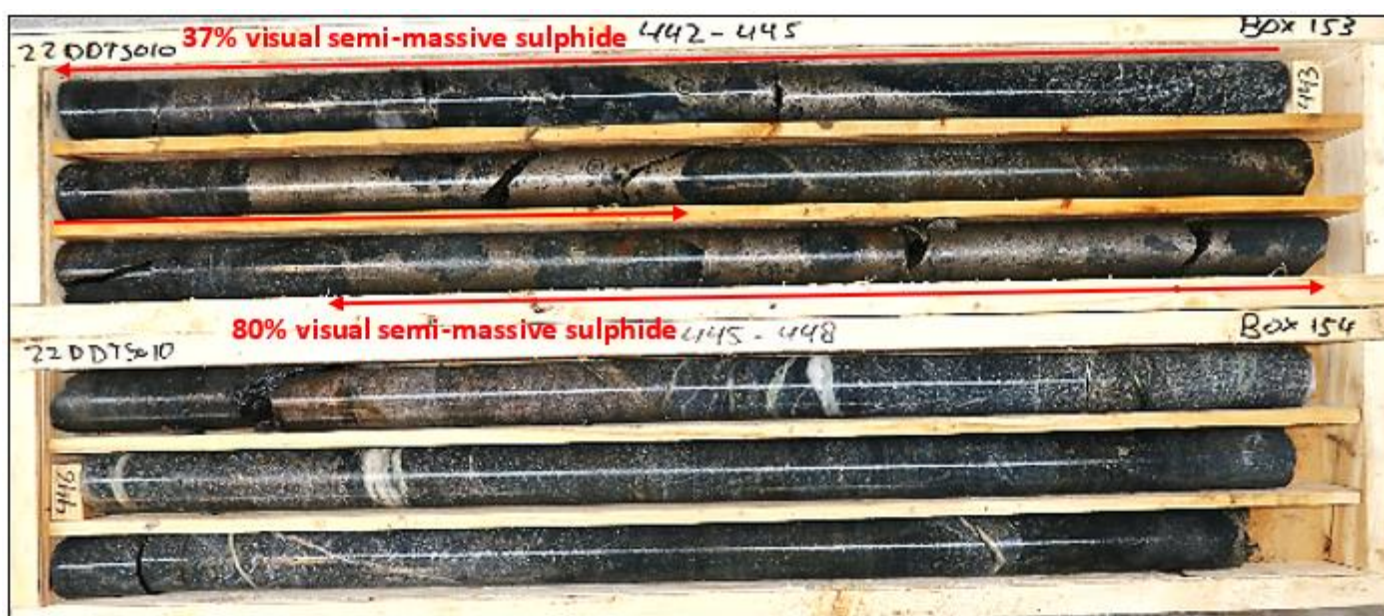
Figure 1: Semi-massive sulphides in the base of hole 22DDTS010 (442m-448m shown)
