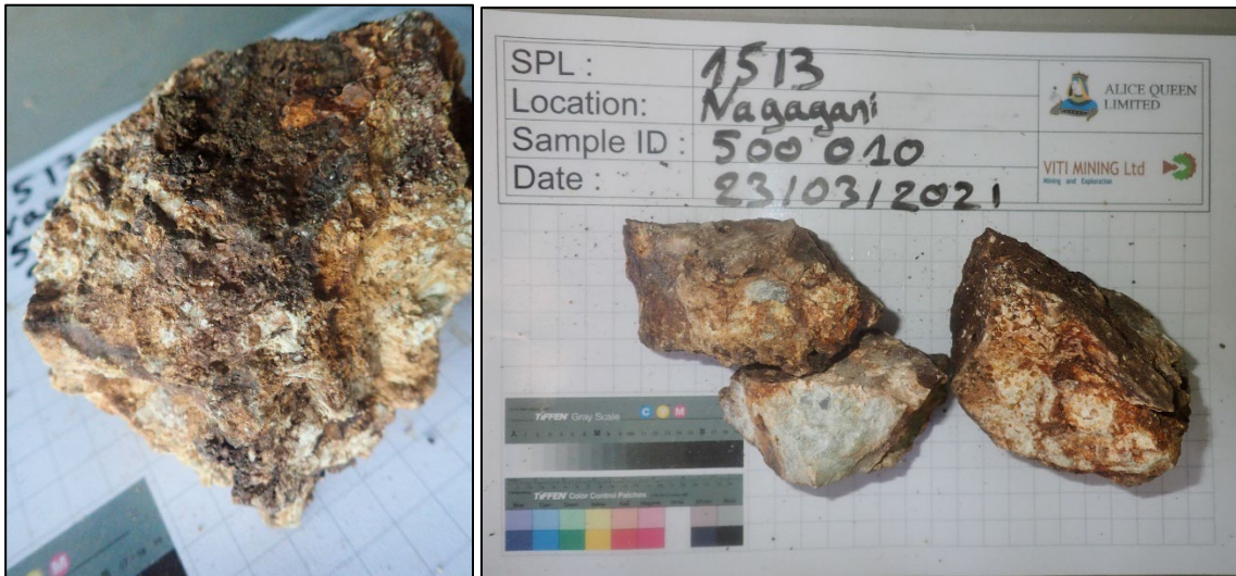
Figure 3 - Weathered rock chip samples (alteration and vein) recently collected from the Nagagni and Karikarimasi creek area (Dakuniba Prospect, SPL1513) returning 4.6g/t Au (left) and 1.4 g/t Au (right) collected from an earlier reconnaissance trip.
