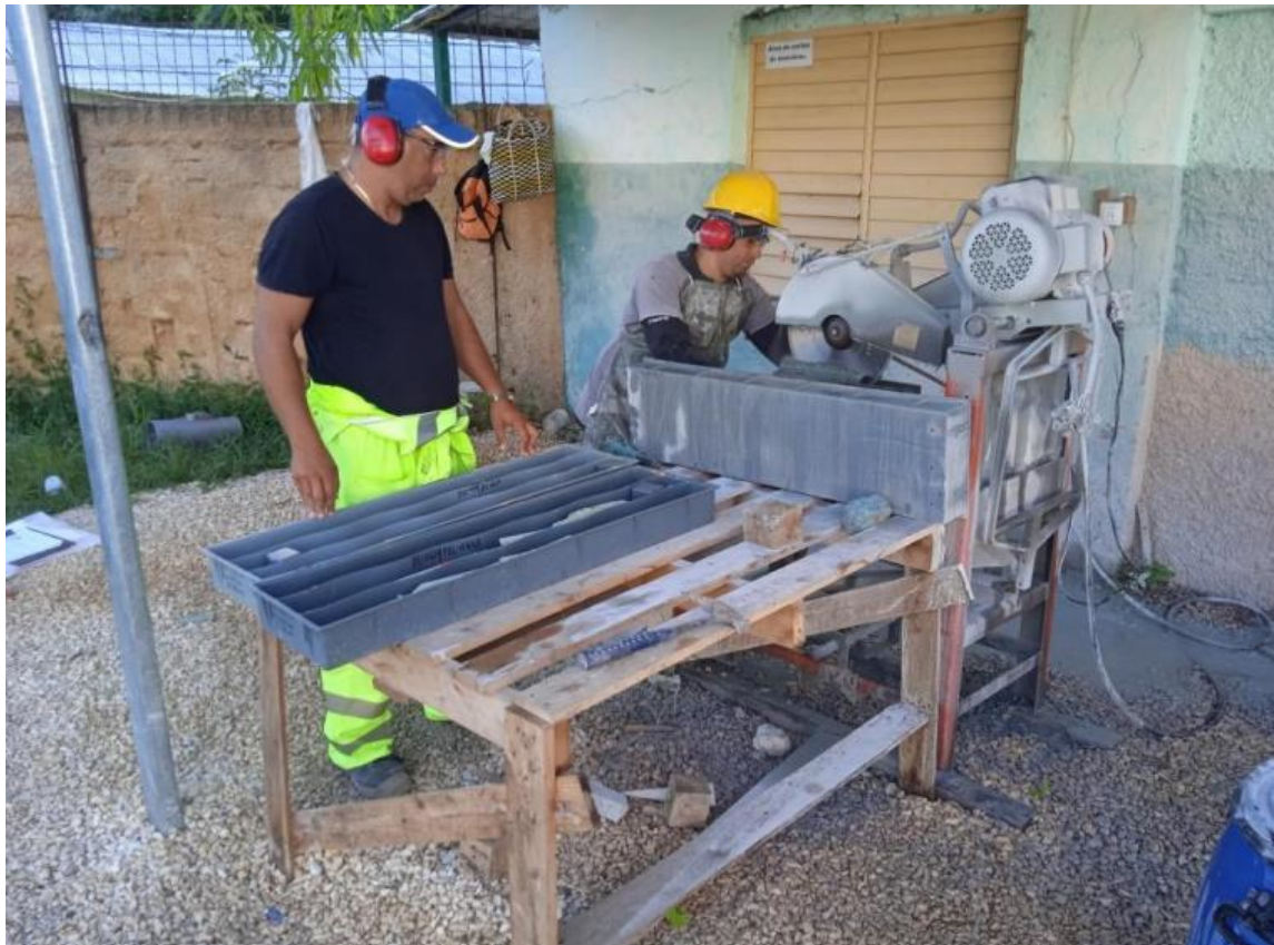
Splitting Cores for Assays
