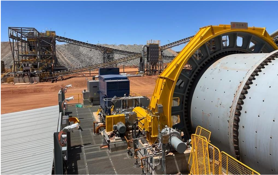
Figure 9 – Ball mill circuit with crushing circuit in the background (Photo 11 November).
