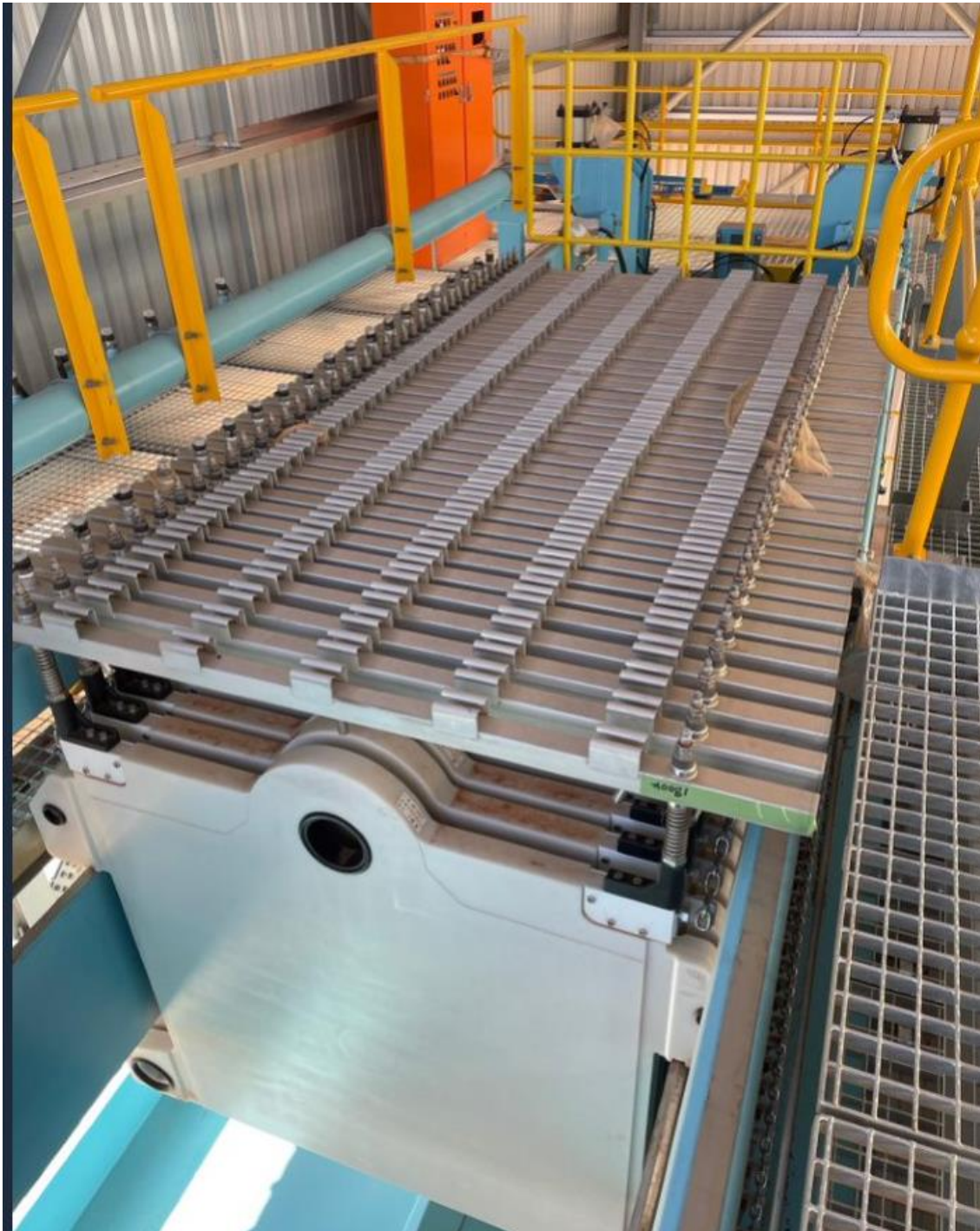
Figure 13 – Concentrate shed filter press.
