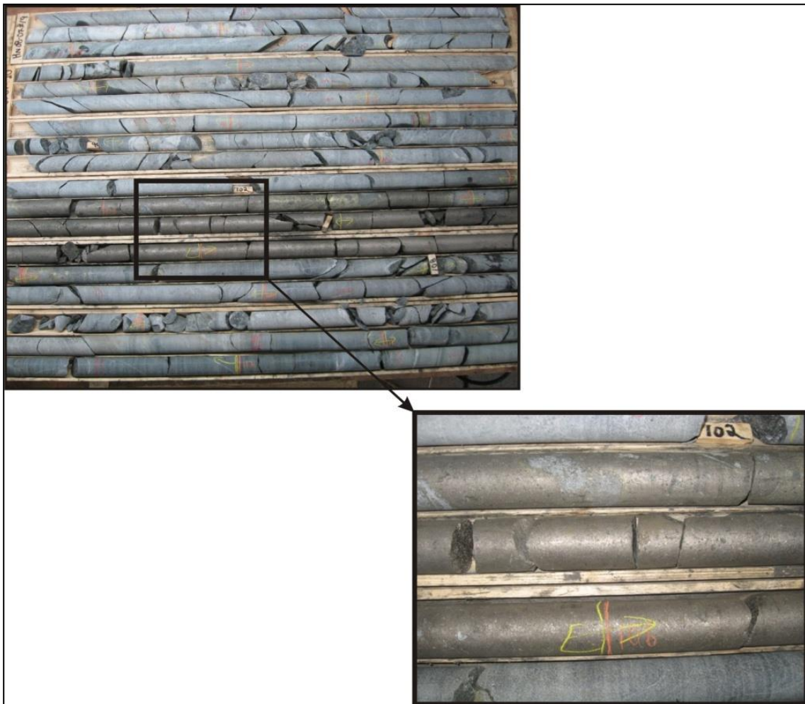
Figure 8. Photograph of drill core from hole HN-08-07 (102.71-107.00 m) from Southampton's 2008 drilling program showing large blebs of pyrrhotite, pyrite and chalcopyrite and massive sulphide in a shear zone at the contact between gabbro and metasedimentary rocks. Drill core diameter is 47.6 millimetres (Kelso et al., 2011). Assay data returned 2.48% Cu, 0.91% Ni, 0.51ppm Pd and 0.26ppm Au over 4.29m for the interval starting at 102.71m.
