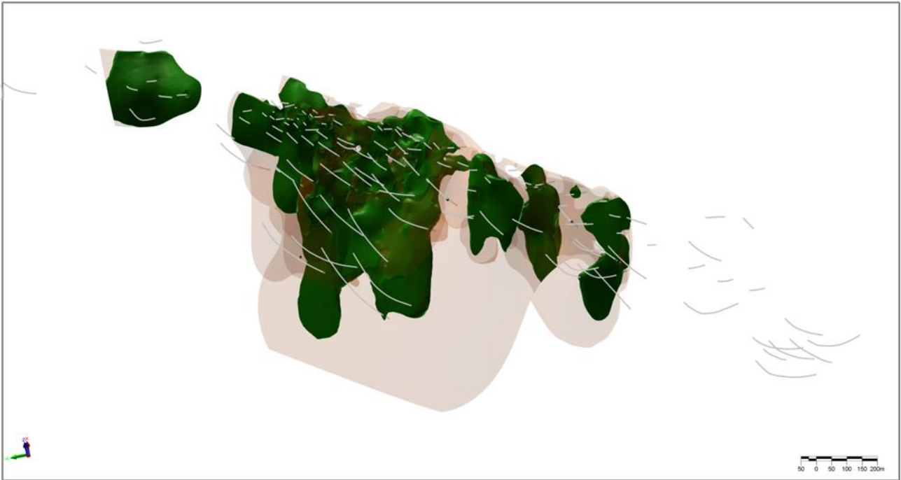
Figure 11. Wireframed domains for copper (transparent orange) and nickel (green), showing their relative spatial distribution within the mineralized zone.
