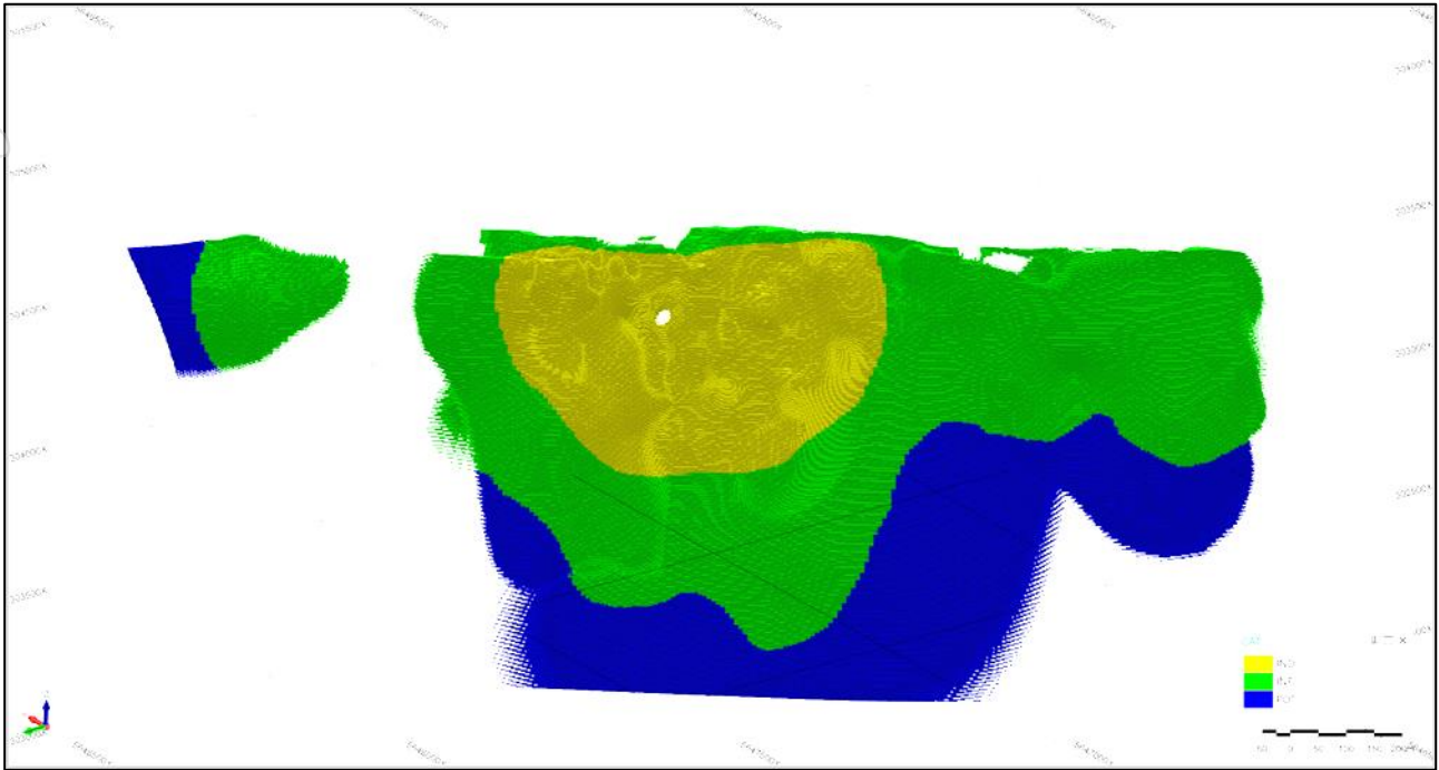
Figure 16. Classification of the resources as Indicated (yellow) and Inferred (green) with unclassified blocks (blue) representing the exploration target potential.
