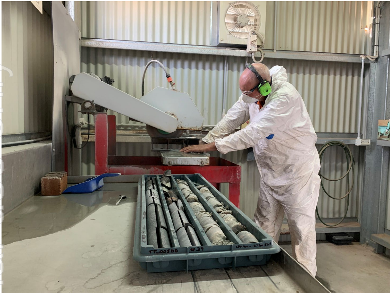
FIGURE 5: CUTTING CORE FROM TT_005DD
