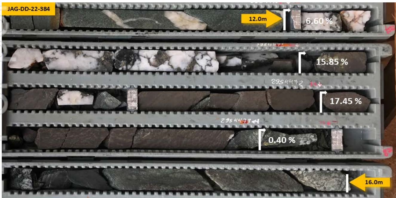
Figure 5 – JAG-DD-21-384 (Jaguar North), 12.0m to 16.0m: Semi-massive to massive sulphides (dark metallic bronze) mineralisation with magnetite alteration (black) hosted in basement gneiss. This interval returned 4.0m at 9.22% Ni, 0.19% Cu and 0.24% Co from 12.0m
