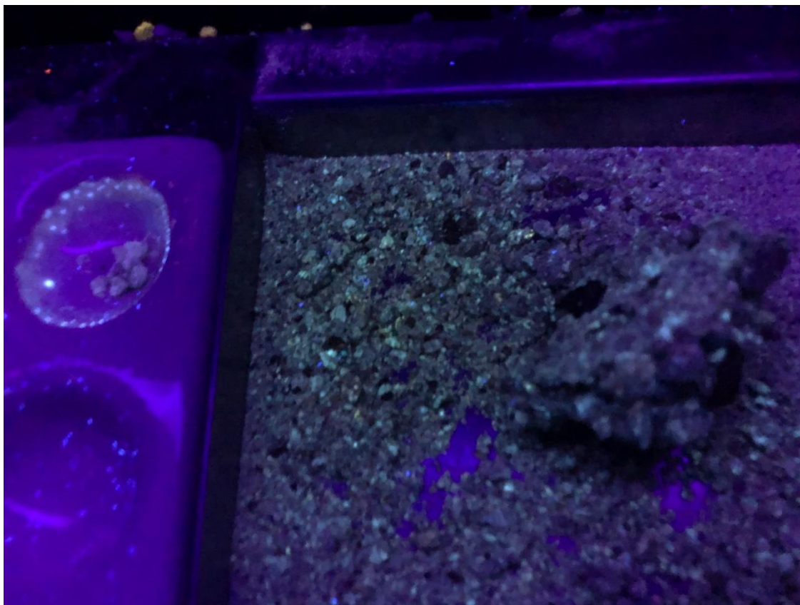
Figure 1 - Cuttings sample from ~3070m MD showing fluorescence (50% following several hours from initial sampling) and residual ring
