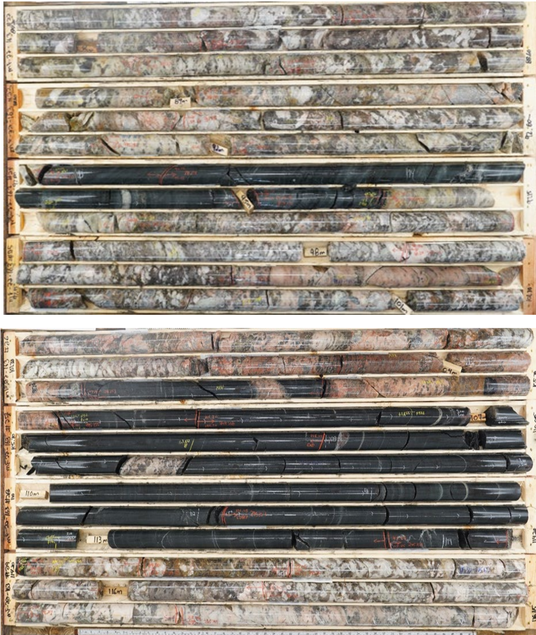
Figure 1 – MF22-163 core photo from 80.05 to 101.3m depth (top image) and from 101.4 to 118.65m depth (bottom image) showing significant spodumene mineralisation throughout the pegmatites.
