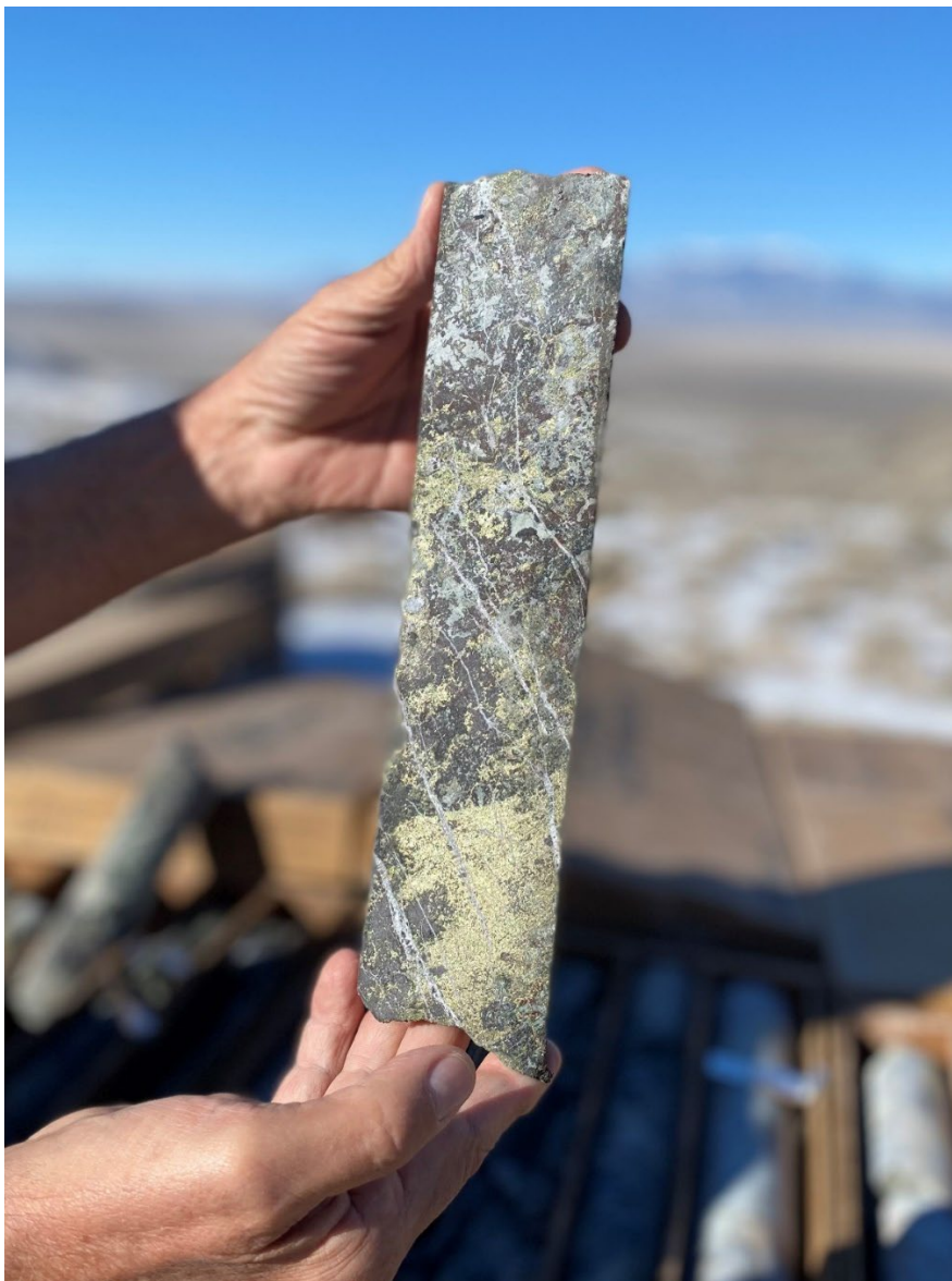
Figure 1: Indium rich chalcopyrite and sphalerite in drill core from WD22-01C (approx. 418m downhole)
