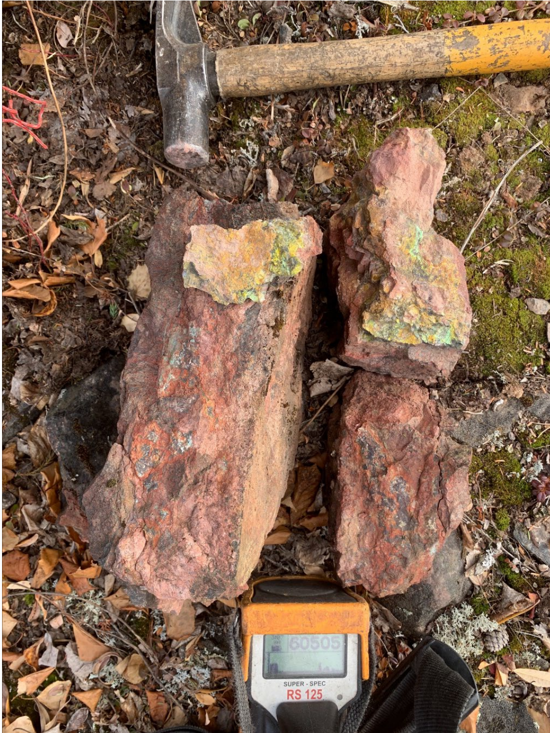
Figure 4: Uranium mineralisation in hematitic breccia from Surprise Creek Fault target
