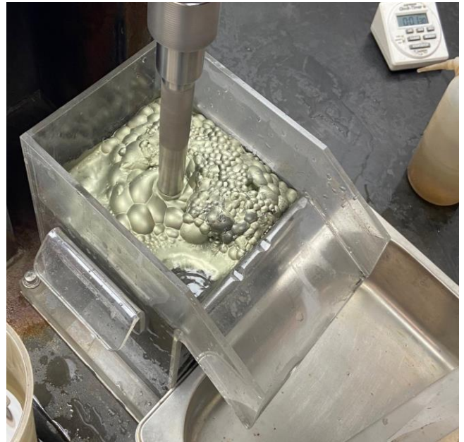
Figure 2: Flotation testwork underway on C3 bulk composite sample. Zinc re-cleaner with chocolate coloured froth (lefthand side) and Copper and Lead cleaner cell with green/gold froth (righthand side)
