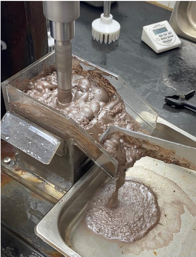
Figure 2: Flotation testwork underway on C3 bulk composite sample. Zinc re-cleaner with chocolate coloured froth (lefthand side) and Copper and Lead cleaner cell with green/gold froth (righthand side)
