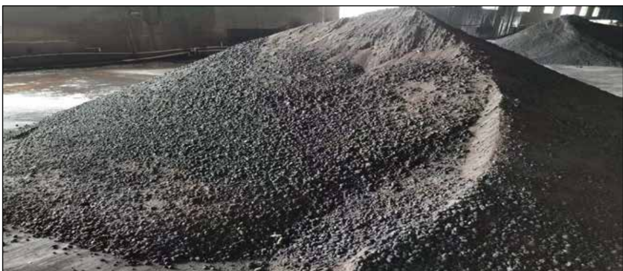
Figure 9 – Mixed material from Scheme 2 ready for smelting. Source: Jiuxing and Nanjing Radiant International
