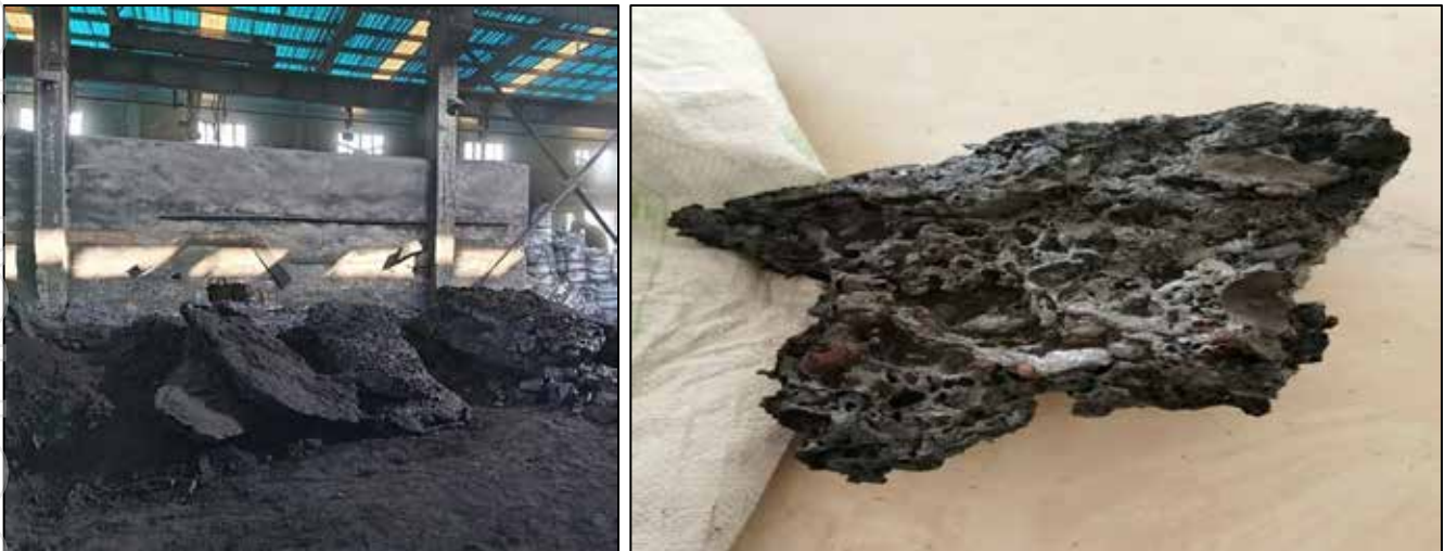
Figure 1 – Left – Titanium chloride grade slag produced from the smelting trials; Right – Pig iron produced from the smelting trials. Source: Jiuxing.
