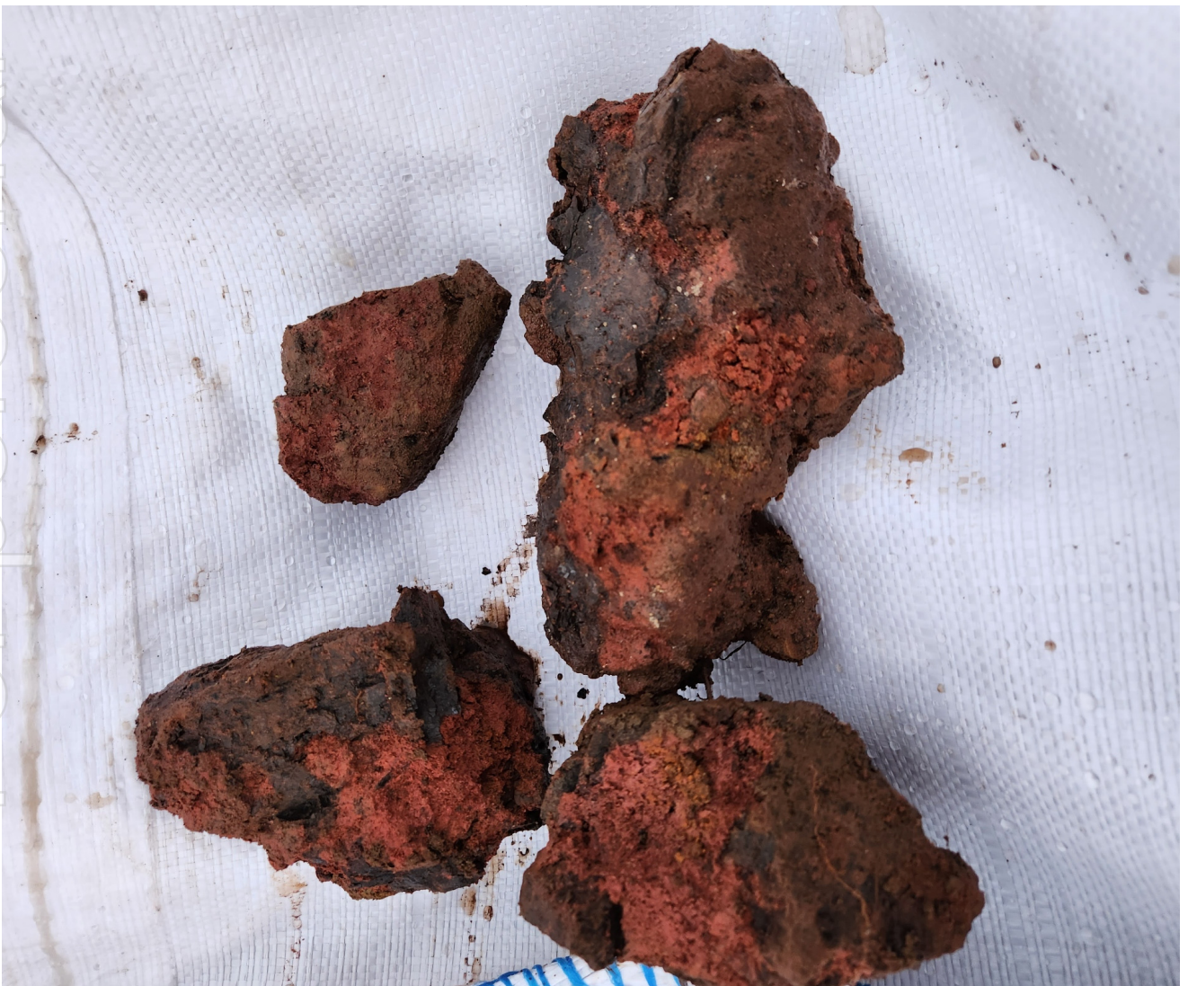
Figure 5: Trench samples showing altered dolerite dyke with pink mineral and highly altered carbonatite with magnetite (similar to samples sent to St Andrews University).
