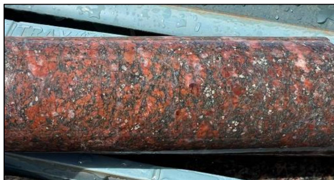
Figure 8: Pervasive iron oxide staining (red) together with hematite (grey) minor magnetite and sericite alteration of the host granite (HELIOS_DD002). NQ drill core \phi ~47mm.
