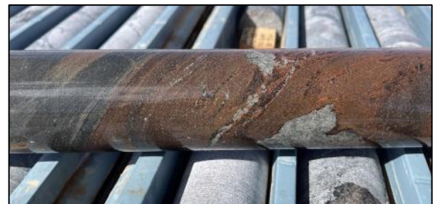
Figure 13: Photo of HQ diamond drill core CENTRAL_DDHC003 showing hematite staining of country rocks.
