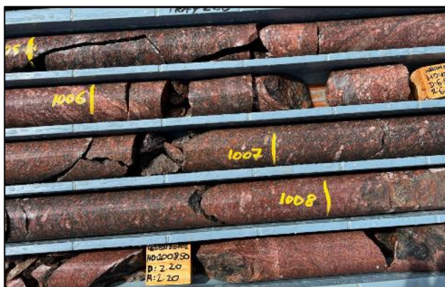
Figure 7: Felsic intrusive breccia containing significant hematite alteration with hematite and minor magnetite and pyrite within the matrix (HELIOS_DDH002). NQ size drill core. Yellow numbering represents down-hole depth in meters.
