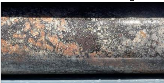
Figure 12: Photo showing an example of granite found in drill core from Central DDHC003.
