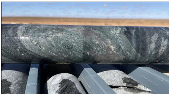
Figure 10: Initial first-pass observation of stage 2 hydrothermal alteration of host rocks. Initial observations indicate epidote-chlorite-sericite +/- actinolite and biotite alteration. Diamond HQ drill core Central_DDHC003.
