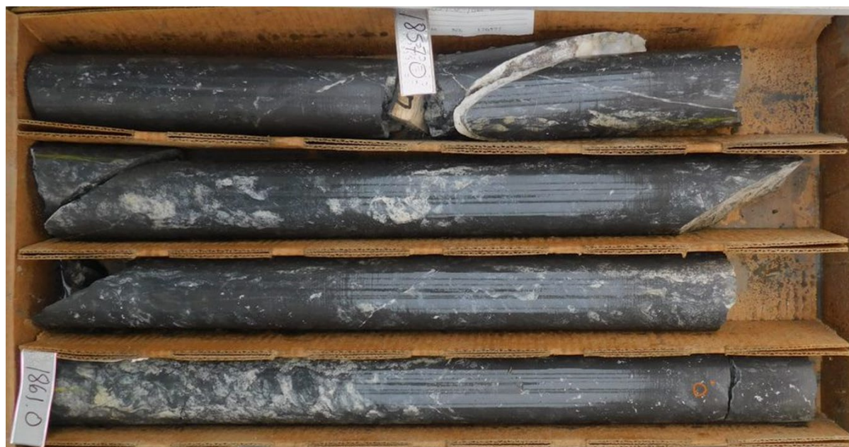
Figure 5: Photo of massive sphalerite (zinc sulphide – black/brown) and magnetite (black) in drill hole WD22-05 at approximately 566 – 567.2m (1857 – 1861ft) downhole.
