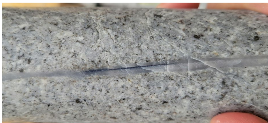
Figure 2: Molybdenite within quartz vein in drill core from WD22-01C at approximately 744.29m (2442ft).
