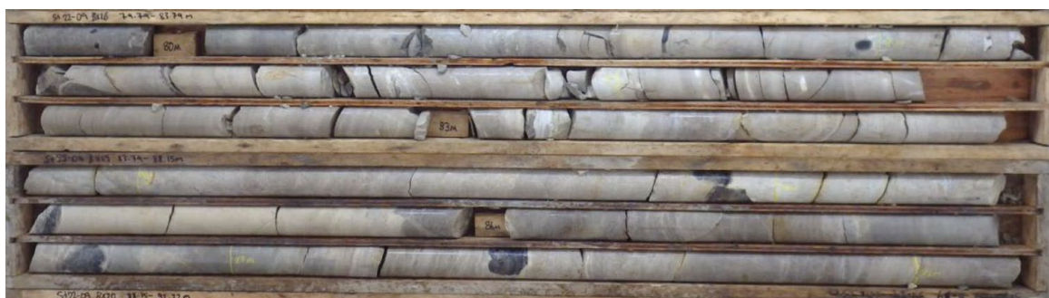
Figure 20: Drill core from ST22-09 between 79.79–88.15m downhole with dark grey chalcocite veining.
