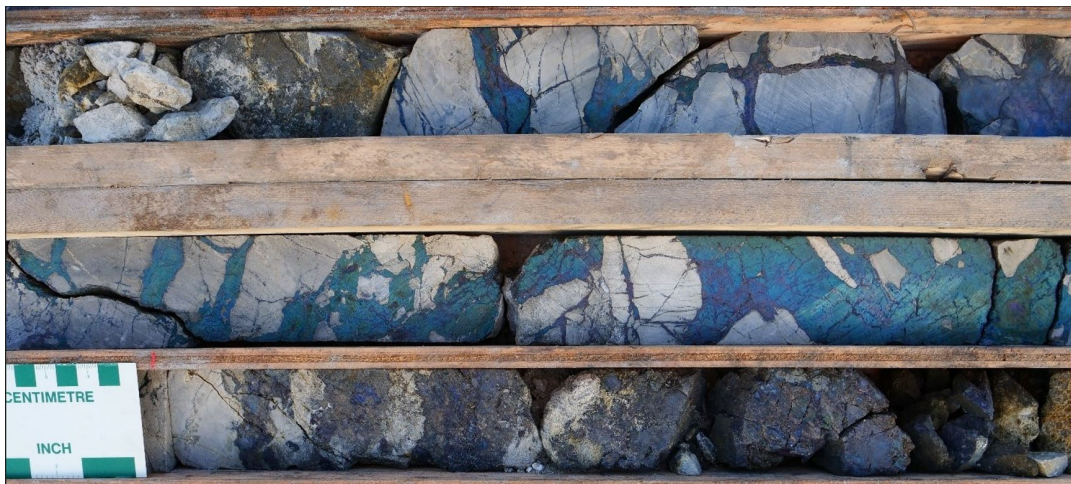
Figure 19: Massive and fracture-fill bornite and chalcocite from approx. 50m downhole in ST22-05.
