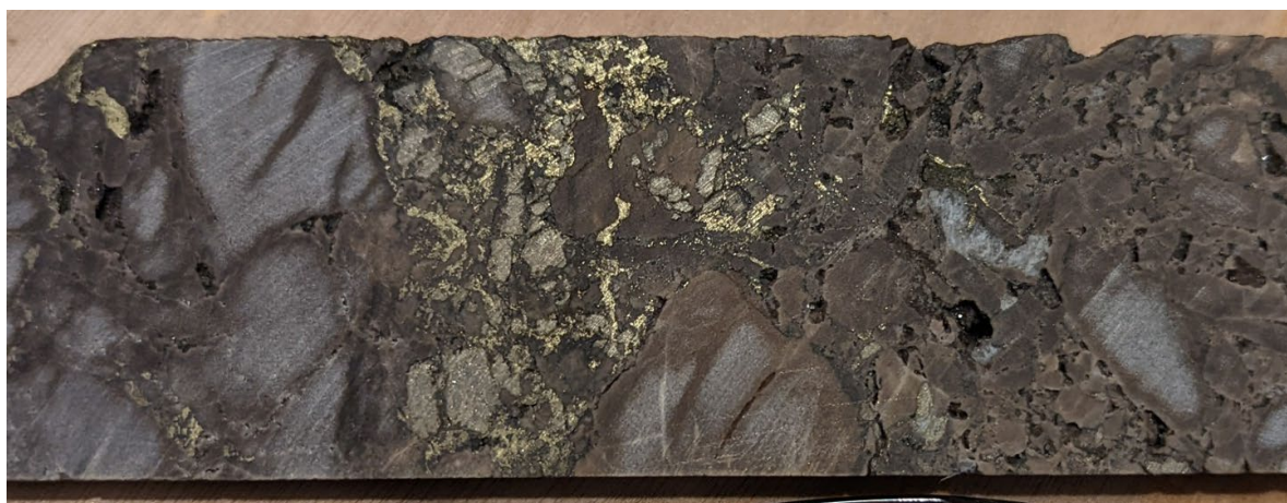
Figure 21: Chalcopyrite (copper sulphide) within ST22-10 drill core from 313m downhole.
