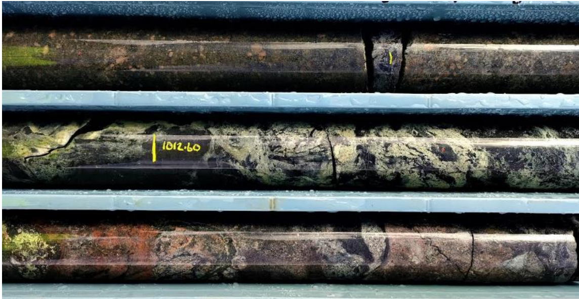
Figure 8: Chalcopyrite encountered in HWDD08 at 1,012m.
