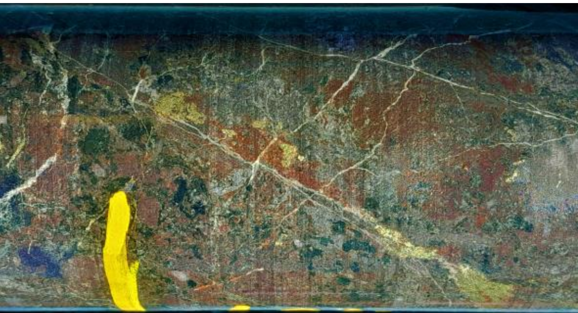
Figure 7: HWDD07 1157m. Vein and disseminated chalcopyrite in altered mafic intrusive in the footwall of the upper Bluebush Fault.
