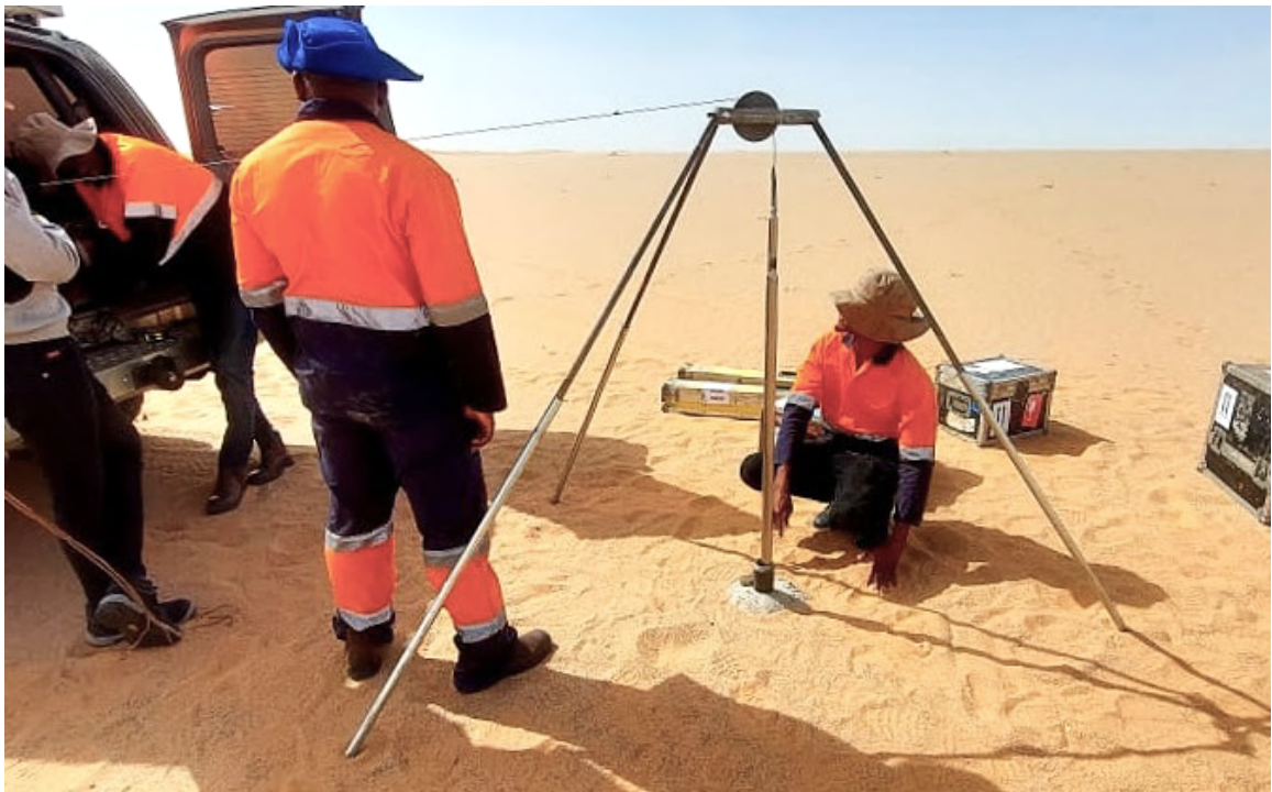
Figure 11 – Downhole gamma logging
