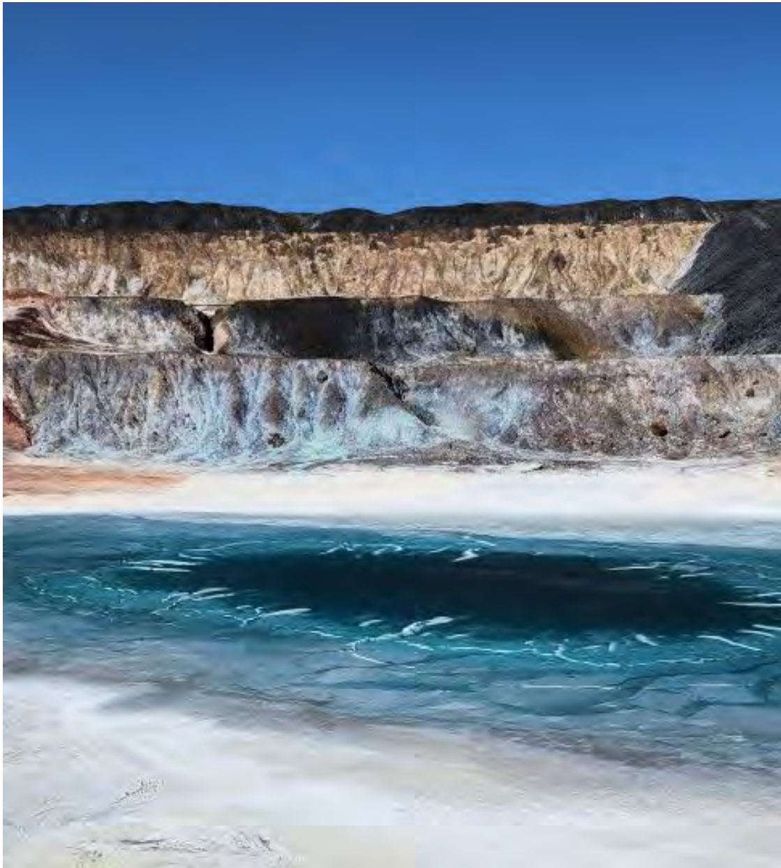
Image 3 / Copper Leaching from Heaps – blue is copper sulphate
