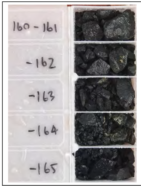
Image 13 / RC drill chips: 22SKRC001 146m to 165m, Gabbro with stringer pyrrhotite/pyrite/chalcocopyrite. 19m at 5,000 ppm Cu, 1,297 ppm Ni, 100 ppm Co, 0.28 ppm Pd, 0.11 ppm Pt
