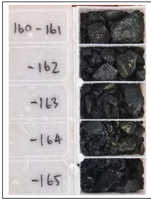
Image 13 / RC drill chips: 22SKRC001 146m to 165m, Gabbro with stringer pyrrhotite/pyrite/chalcocopyrite. 19m at 5,000 ppm Cu, 1,297 ppm Ni, 100 ppm Co, 0.28 ppm Pd, 0.11 ppm Pt
