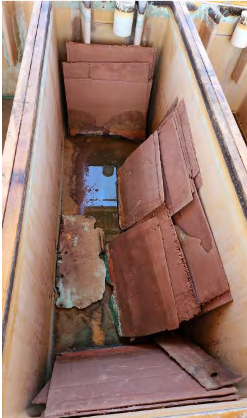
Image 6 / Copper cathode to be recovered from the bottom of an EW cell after removing cathodes and anodes – red metal plates
