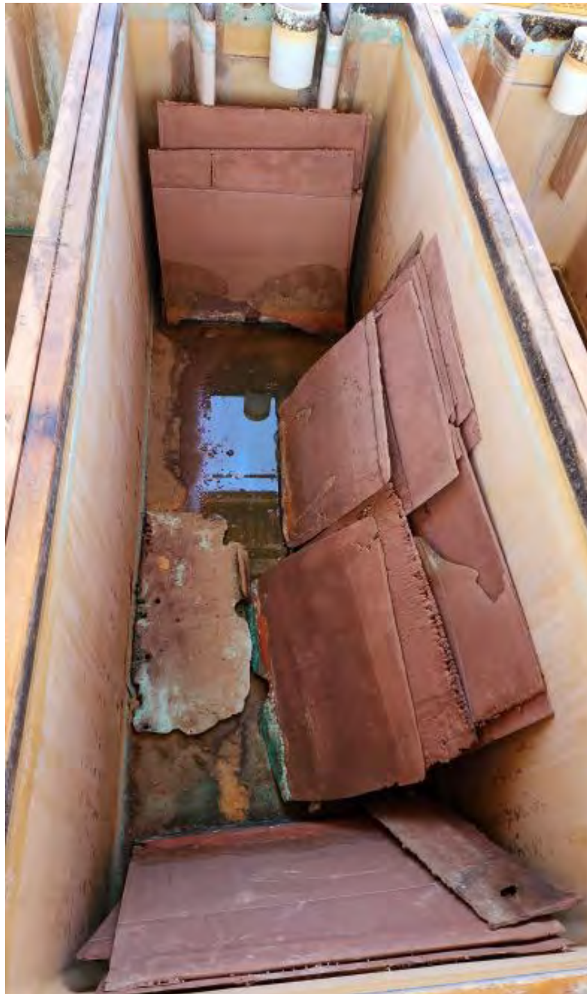
Image 6 / Copper cathode to be recovered from the bottom of an EW cell after removing cathodes and anodes – red metal plates
