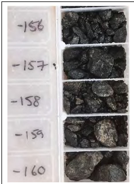
Image 13 / RC drill chips: 22SKRC001 146m to 165m, Gabbro with stringer pyrrhotite/pyrite/chalcocopyrite. 19m at 5,000 ppm Cu, 1,297 ppm Ni, 100 ppm Co, 0.28 ppm Pd, 0.11 ppm Pt
