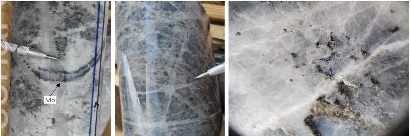
Plate 1. Left: CRDD22-001 (494m) Diorite porphyry with phyllic alteration, 1-2% disseminated chalcopyrite, 2-3% pyrite, 1-2% molybdenite in B-type quartz vein, intensive > 5% quartz veinlet stockwork. Middle: CRDD22-001 (530m) Andesite with potassic alteration, 2-3% disseminated pyrite, trace < 1% chalcopyrite, trace < 1% molybdenite, intensive > 5% quartz veinlet stockwork. Right: CRDD22-002 (94m) Diorite Porphyry with phyllic alteration, 0.5-1% disseminated chalcopyrite, 2-3% pyrite, 0.5-1% molybdenite in B-type veins.
