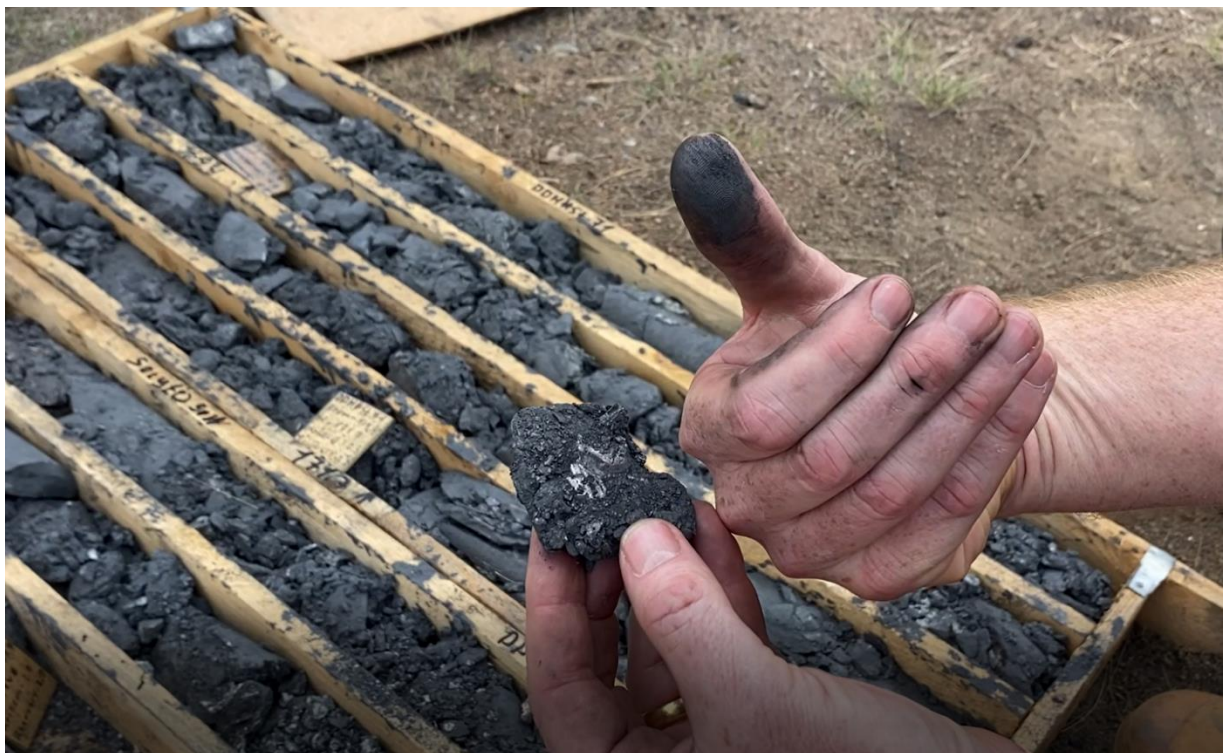
Figure 2 - High-grade graphite at 170m in ST-71 to the north-east of the CGZ
