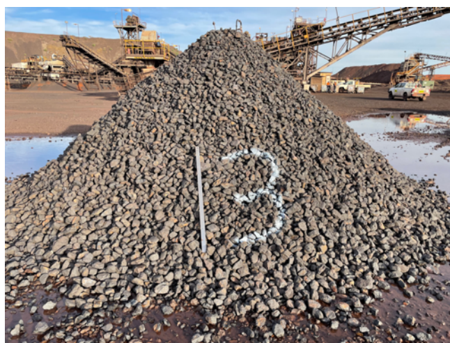
Figure 14. Butcherbird ore post DMS processing
