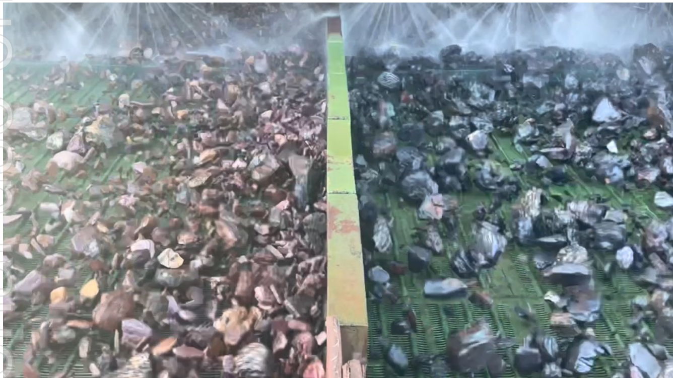
Figure 12. Butcherbird feed material on the wash screen after densimetric separation showing a clear delineation product and waste.
