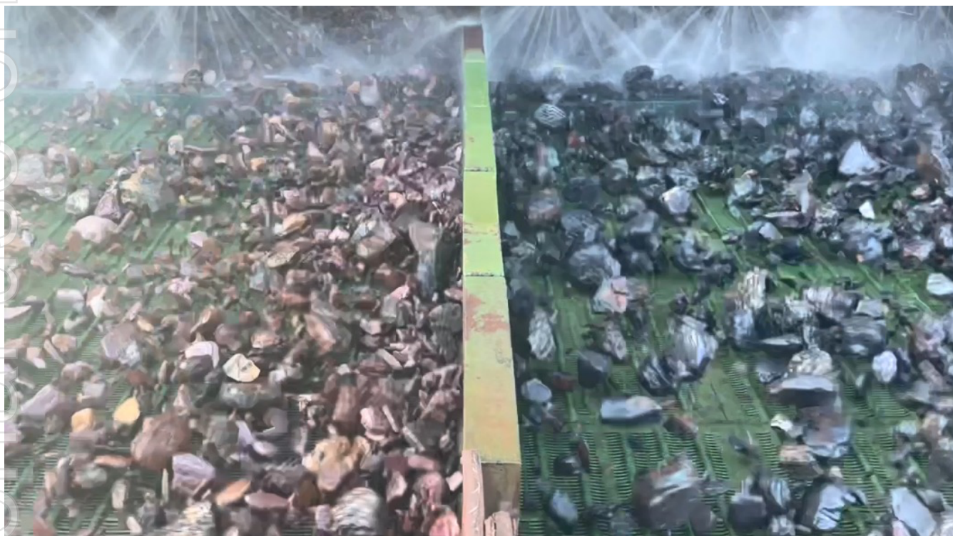
Figure 12. Butcherbird feed material on the wash screen after densimetric separation showing a clear delineation product and waste.
