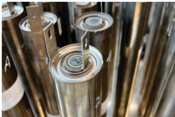
SAS cell with positive and negative terminal individual cell rated at 2.58 V each
