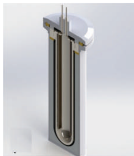
Cross section of CERENERGY® Battery
