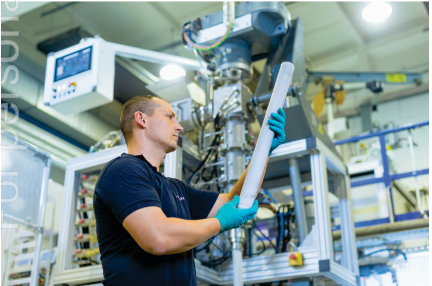
Ceramic solid-state electrolyte at Fraunhofer IKTS pilot facility - SAS cells in battery module
