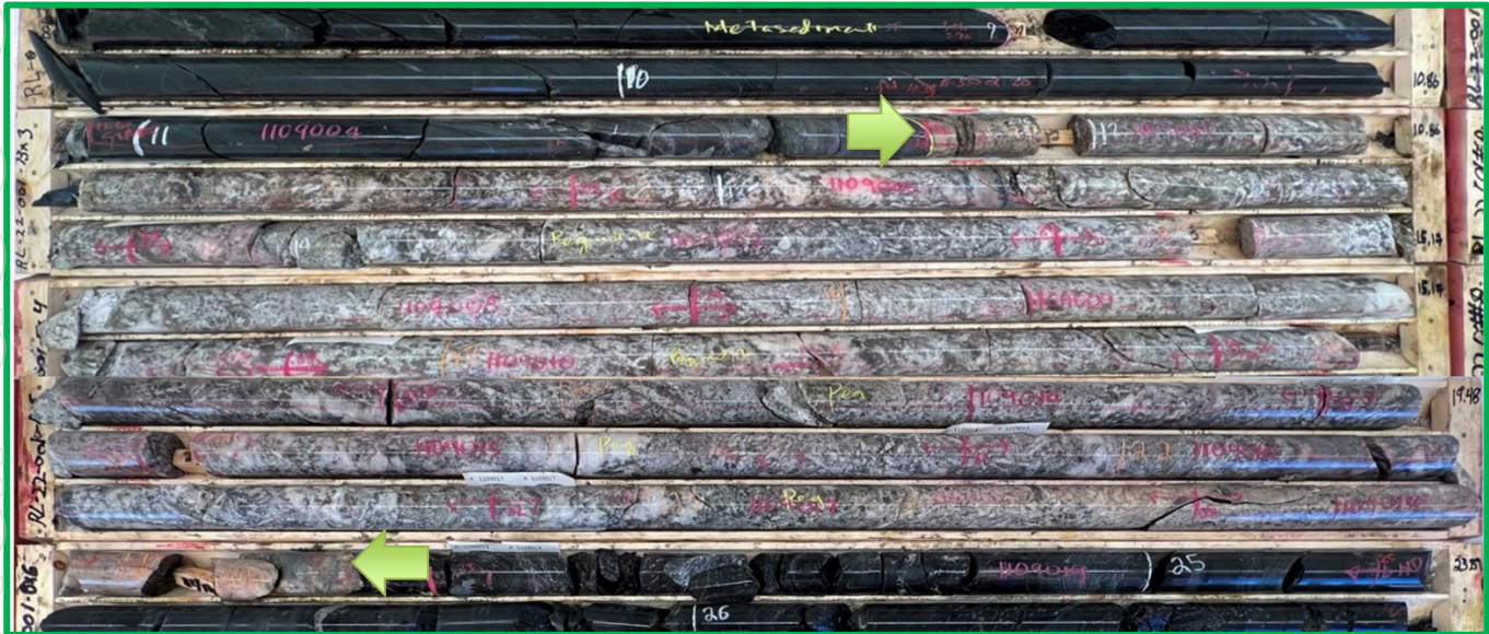
Figure 5: RL-22-001 – Whole NQ Core diamond core showing high density spodumene crystal laths, 12.38m @ 1.85% \text{Li}_2\text{O}
