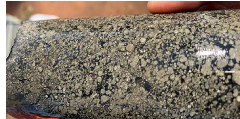
Coarse pyrite in skarn: 0.63g/t gold & 3.4% copper @ 64.1-65m
