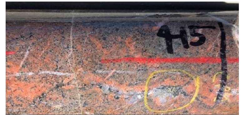
Altered quartz-monzodiorite with quartz-py-cpy veining and vein selvage potassic alteration @ 415m
