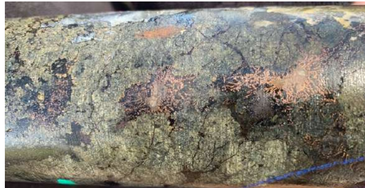
Native copper, chalcocite, chalcopyrite and black chlorite in skarn: 4.24g/t gold & 1.6% copper @ 60.6-61.6m
