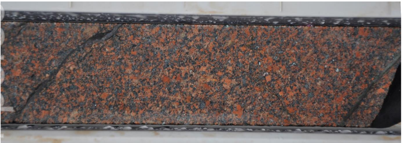
Figure 5: 22MEDD001 magnetite, hematite, albite, sericite, chlorite and epidote alteration in monzodiorite at 702m
