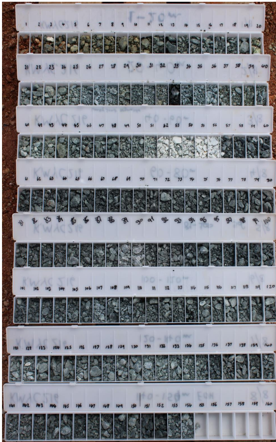
Figure 14 - RC chips for hole KMYC216 drilled directly underneath Lucky Sump where surface spodumene-bearing pegmatite samples returned up to 1.91% Li 2 O. Note the white chips in metres 52-56m. Results pending
