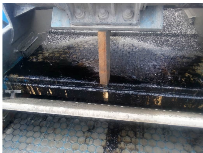
Figure 3 - Free oil on shakers (Zapato-1)
