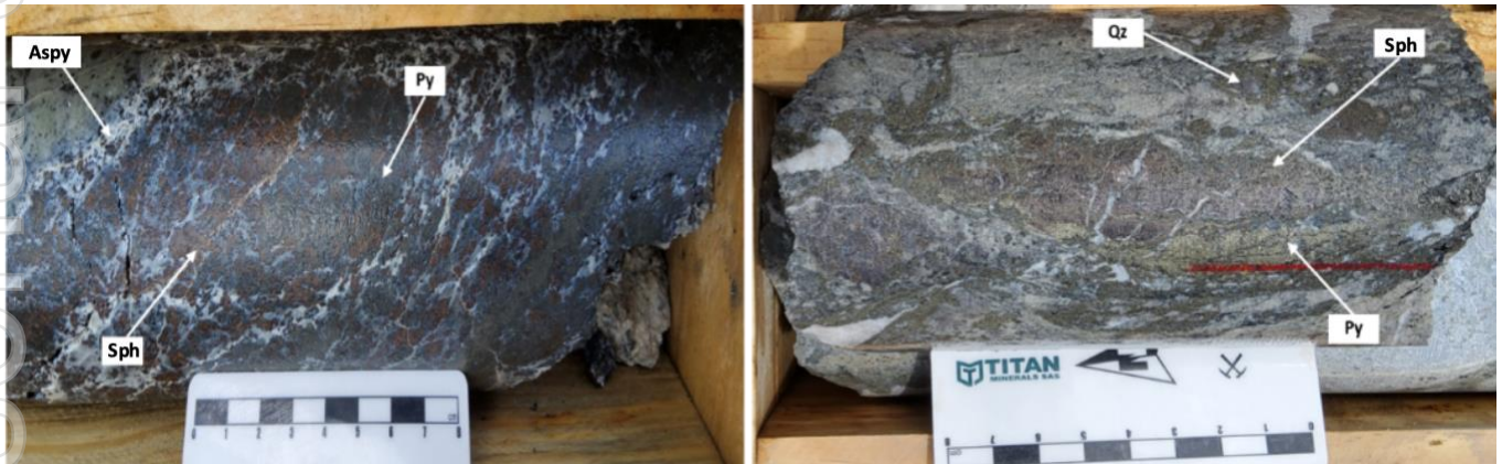
Plate 1: Diamond core from Meseta Gold prospect. Left: MGDD22-005 (73.65m) Massive sulphide vein, disseminated mineralisation, 80% pyrite (Py), 10-12% sphalerite (Sph) and 1% arsenopyrite (Aspy) Right: MGDD22-005 (80.75m) Hydrothermal Breccia, disseminated mineralisation, 10-15% pyrite (Py), 2-3% sphalerite (Sph), sub-angular to sub-rounded clasts, matrix of sulphides, veinlets of calcite, quartz (Qz) vein with comb texture.
