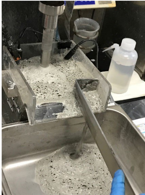
Image 5: Initial floatation test work study Source: Temarise/ ALS Labs Perth
