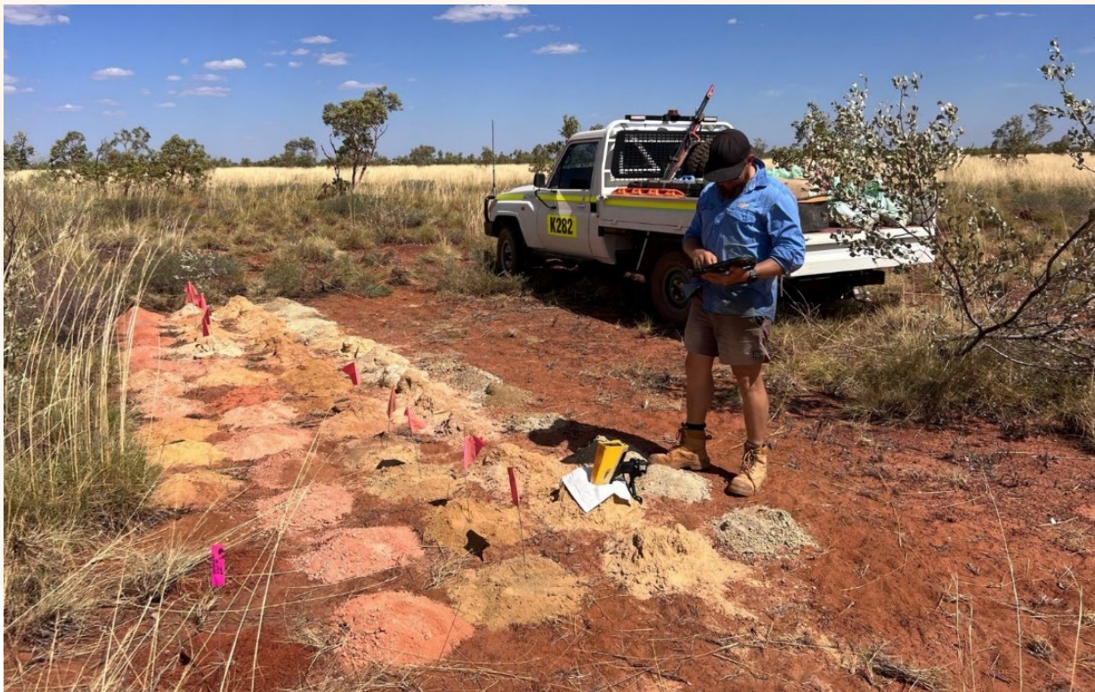
Figure 1: pXRF testing regional air-core drilling at the Tanami Heavy REE Project, WA. Pink flags represent pXRF yttrium anomalism which is sampled as 1m samples.
