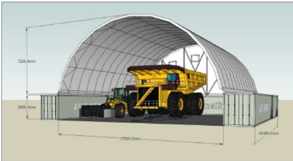
Figure 25: Example of Double-container height Haulpak workshop.
