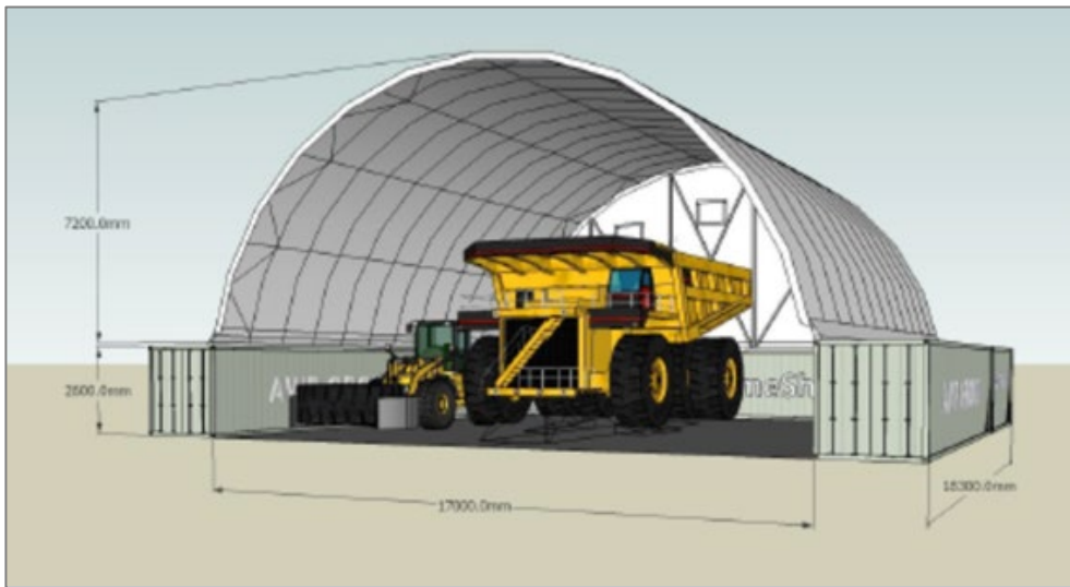
Figure 25: Example of Double-container height Haulpak workshop.
