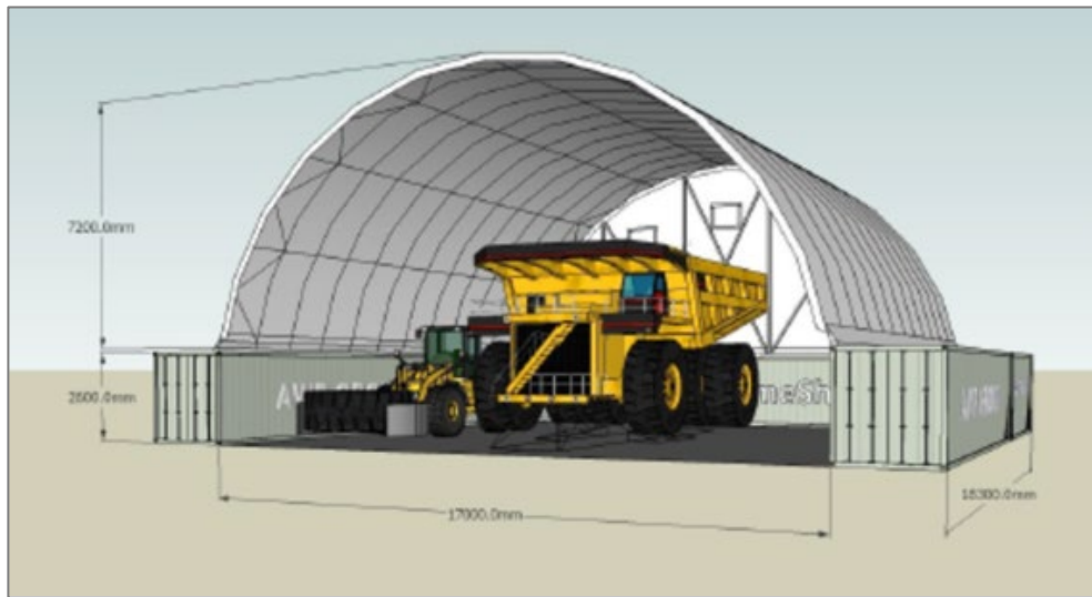
Figure 25: Example of Double-container height Haulpak workshop.
