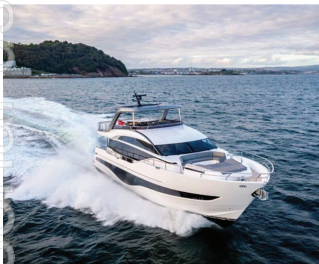
Figure 9: The latest Y85 from Princess Yachts features a pair of 41" VEEMStar-C propellers enabling a top speed of 31 knots.
