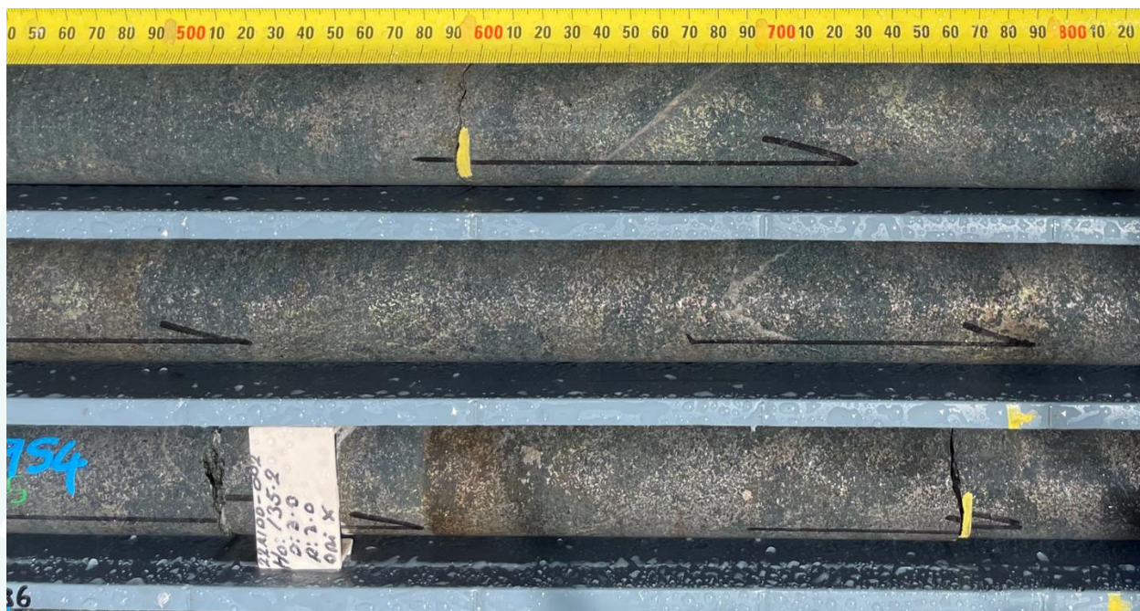
Figure 4: 22A1DD002 (133.5-135.5m interval – NQ core 47.6mm diameter). Mineralised pyroxenite with fine-to-coarse grained disseminated pyrrhotite and chalcopyrite. Within a 15.9 metre zone of sulphide mineralisation. 1
