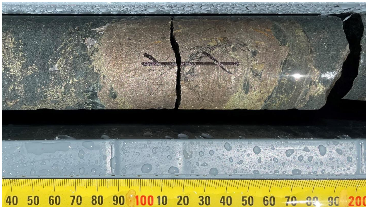
Figure 1: 22B1DD003 (101.3-101.4 metre interval – NQ core 47.6mm diameter). Mineralised dolerite with fine-grained massive pyrrhotite and chalcopyrite, with lesser pentlandite. Within a 22.2 metre zone of sulphide mineralisation. 1
