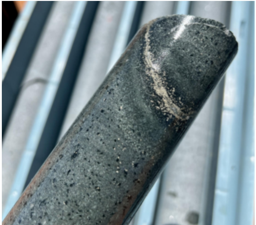
Figure 02: Silica and sulphide (pyrite and pyrrhotite) altered medium grained dolerite with coarse pyroxene phenocrysts at 580m.
