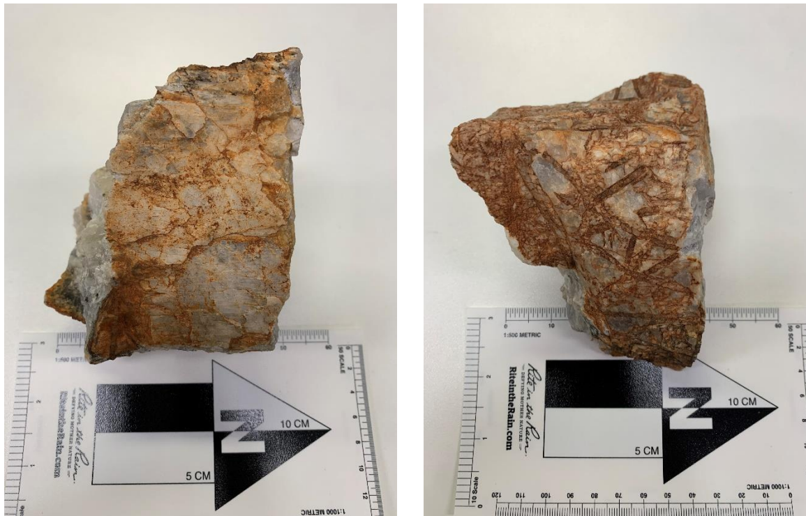
Figure 1: Duplicate of sample APRK00037 (3.32% \text{Li}_2\text{O} assay) – pegmatite contains large spodumene crystals (left photo) and bladed spodumene on the reverse side (right photo)
