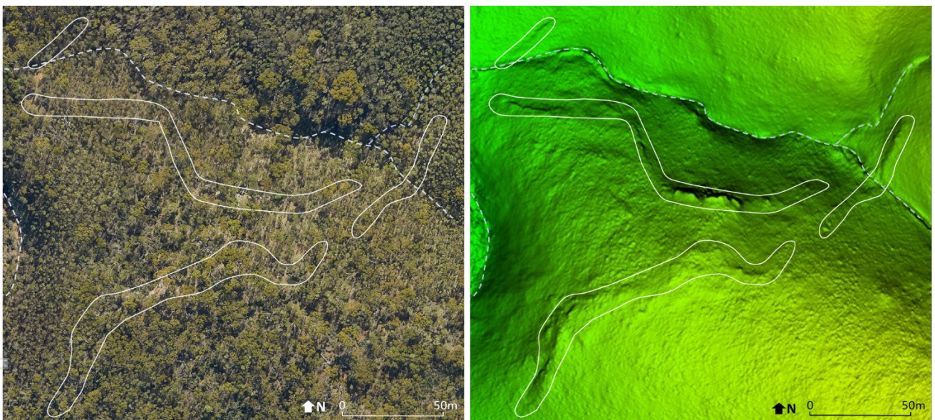
Figure 3: Outlines of verified outcropping pegmatites from on-ground mapping (white outlines) are used for machine learning inputs to generate algorithms for new potential pegmatite targets. Creeks noted as light blue dashes
