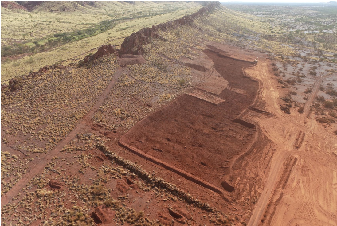
Figure 2: Excavation of Detritals Iron Ore on Northern Slope of Paulsens East Hematite Ridge
