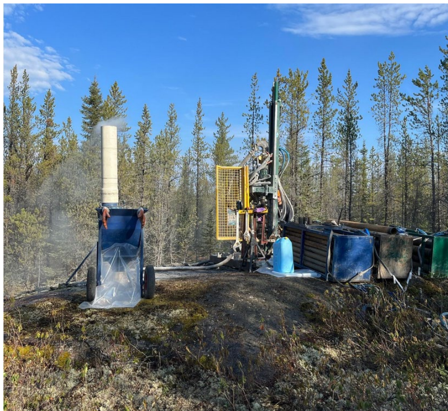
Figure2: RC drill rig assembled for drilling
