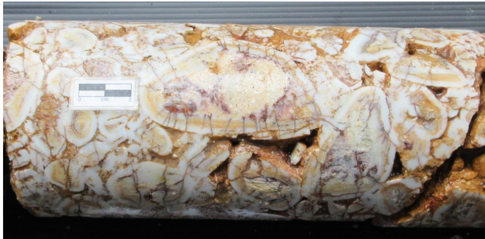
Figure 7: Image of drill core from APD003, 28.6m showing cockade-textured quartz breccia. Such breccia formed during periods of high hydraulic gradient in which quartz accretes over wallrock or pre-existing clasts or fragments. The open-spaced infill character of the breccia is apparent.
