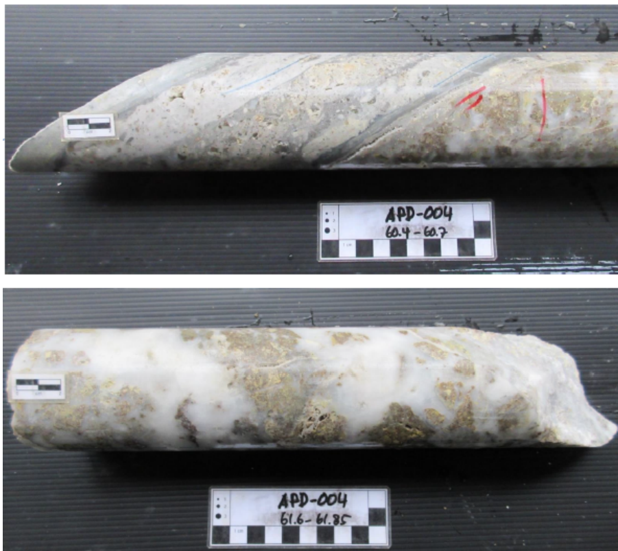
Figure 8: Images of drill core from APD004. These samples show evidence of repeated and superimposed brecciation and quartz veining that occurred within the fault-bounded main zone vein-breccia system.
