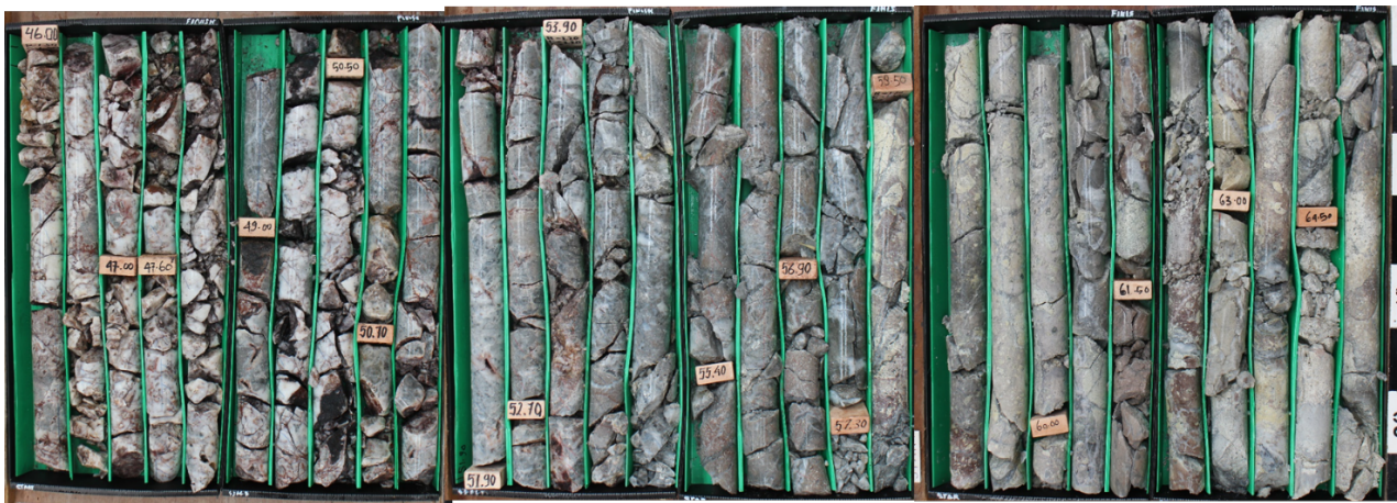
Figure 5: Image of drill core from hole APD002 showing intersection of near massive quartz vein and breccia. The quartz is locally chalcedonic and contains 1-3% of fine-grained disseminated pyrite.
