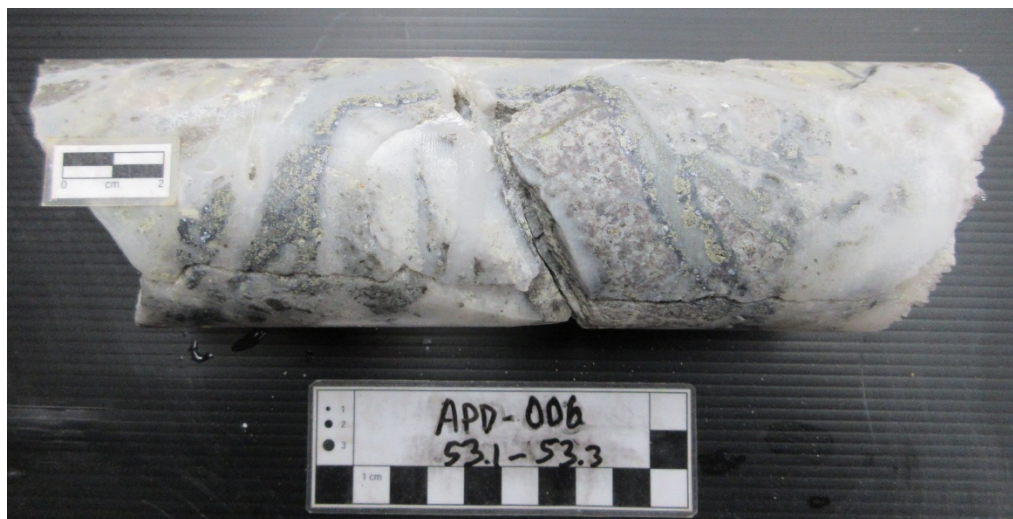
Figure 11: Photograph of quartz breccia in APD006 at 53.1m. The image shows evidence that early brecciation with sulphide mineralization manifests as galena along clast margins. The image indicates that this was followed by later period of brecciation with massive white quartz matrix.
