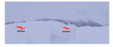
Machine learning and AI based detection and classification software is used to undertake near-real time tracking and assessment of drones and UAS threats
