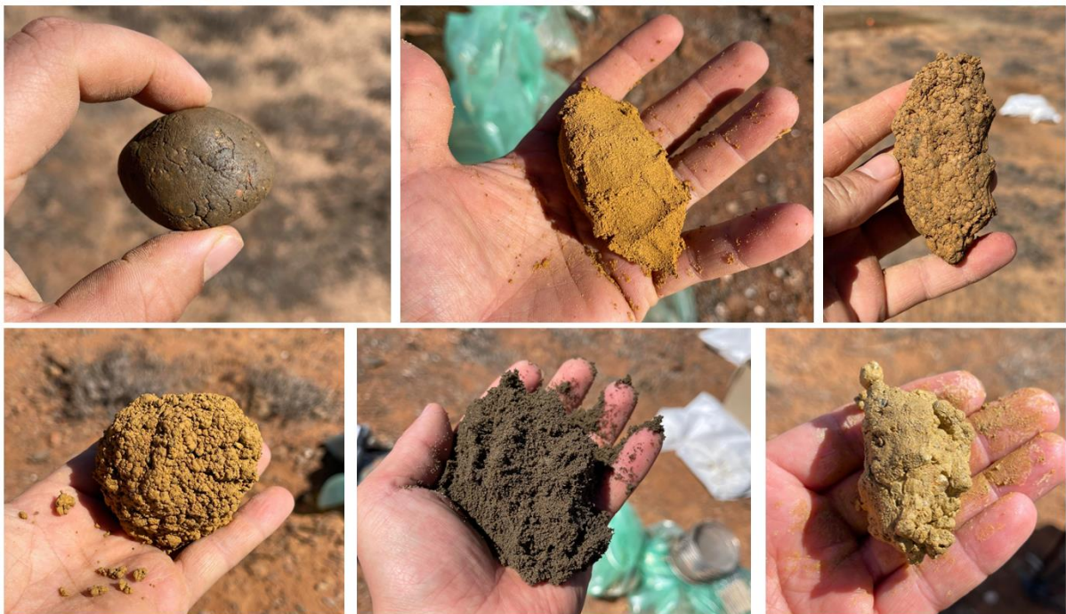
Figure 3. Examples of clays intercepted in the deep weathering profile in multiple RAB drillholes during the recent drilling at Morgans Creek.
