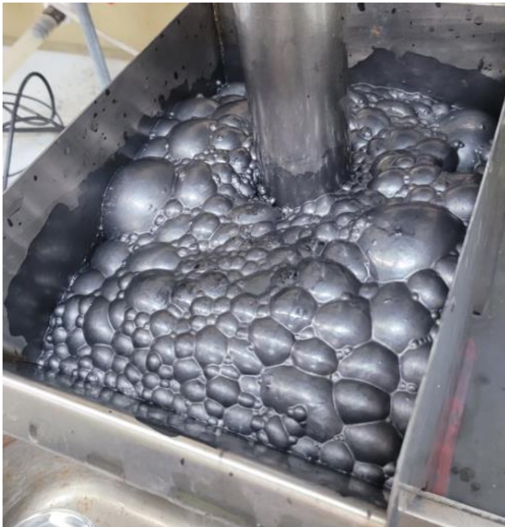
Figure 2 – Flotation test on Sarytogan graphite at the Metallurgy laboratory, Perth
