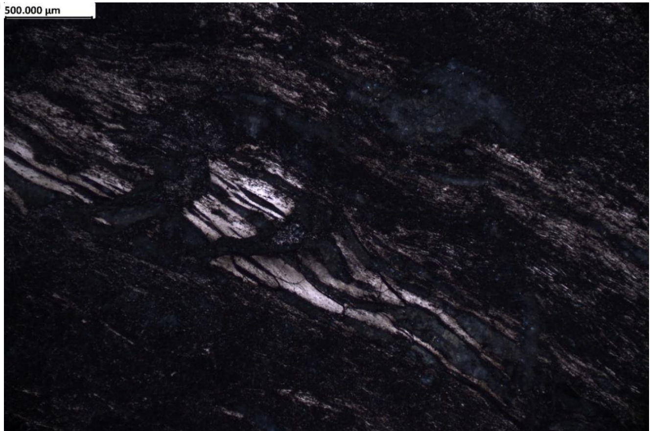
Figure 3 - Thin section photomicrograph of St-47-56.4 (21_1310_209) in reflected light (XPL, 5x objective). Thick graphitic ribbons in graphite schist with late-stage quartz veins crosscutting the fabric.
