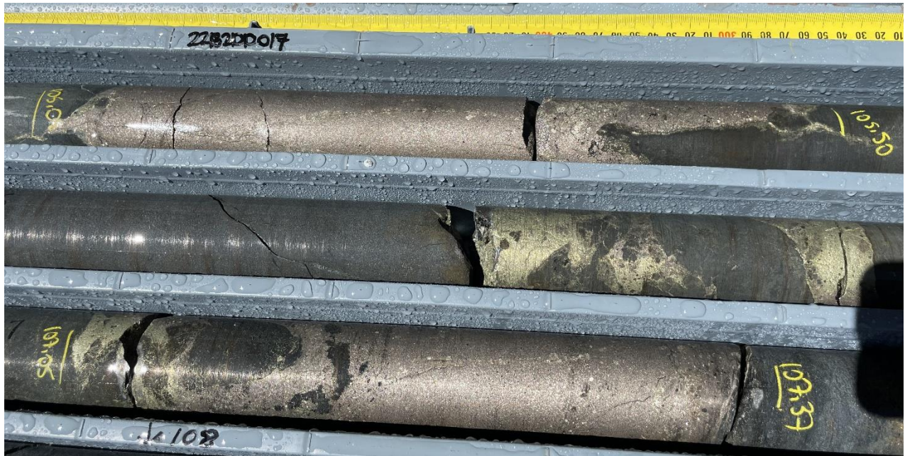
Figure 2: 22B2DD017 (105.08-107.37m interval – NQ core 47.6mm diameter). Strongly mineralised dolerite with bands of fine-grained massive pyrrhotite and coarser pentlandite, along with a zone of chalcopyrite-pyrrhotite-pentlandite. Within a 38.94m zone of sulphide mineralisation. 1
