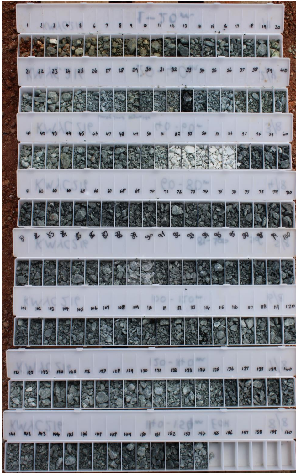
Figure 3. RC chips for hole KMYC216 drilled directly underneath Lucky Sump where surface spodumene-bearing pegmatite samples returned up to 1.91% Li 2 O. Note the white chips in metres 52-56m. Results pending.
