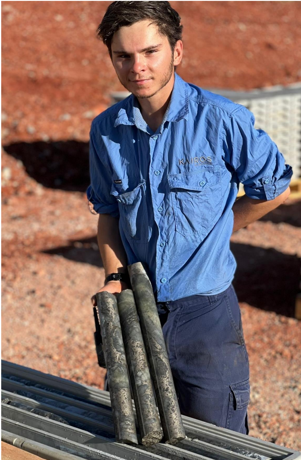
Figure 4. Kairos geologist Will Coussens with core from hole KMYD071 showing extremely silicified and sulphidised (pyrrhotite, pyrite, arsenopyrite) wall rocks at the hangingwall contact of a well mineralised banded iron formation. The mineralisation is typical of the hangingwall sequence and is 15.4m in down-hole thickness at this location at Main Hill prospect (see Figure 5 ).
