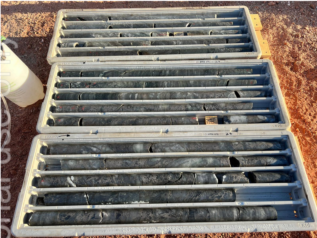
Figure 5. 15.4m of highly silicified-sulphidised core from hole KMYD071 at Main Hill.
