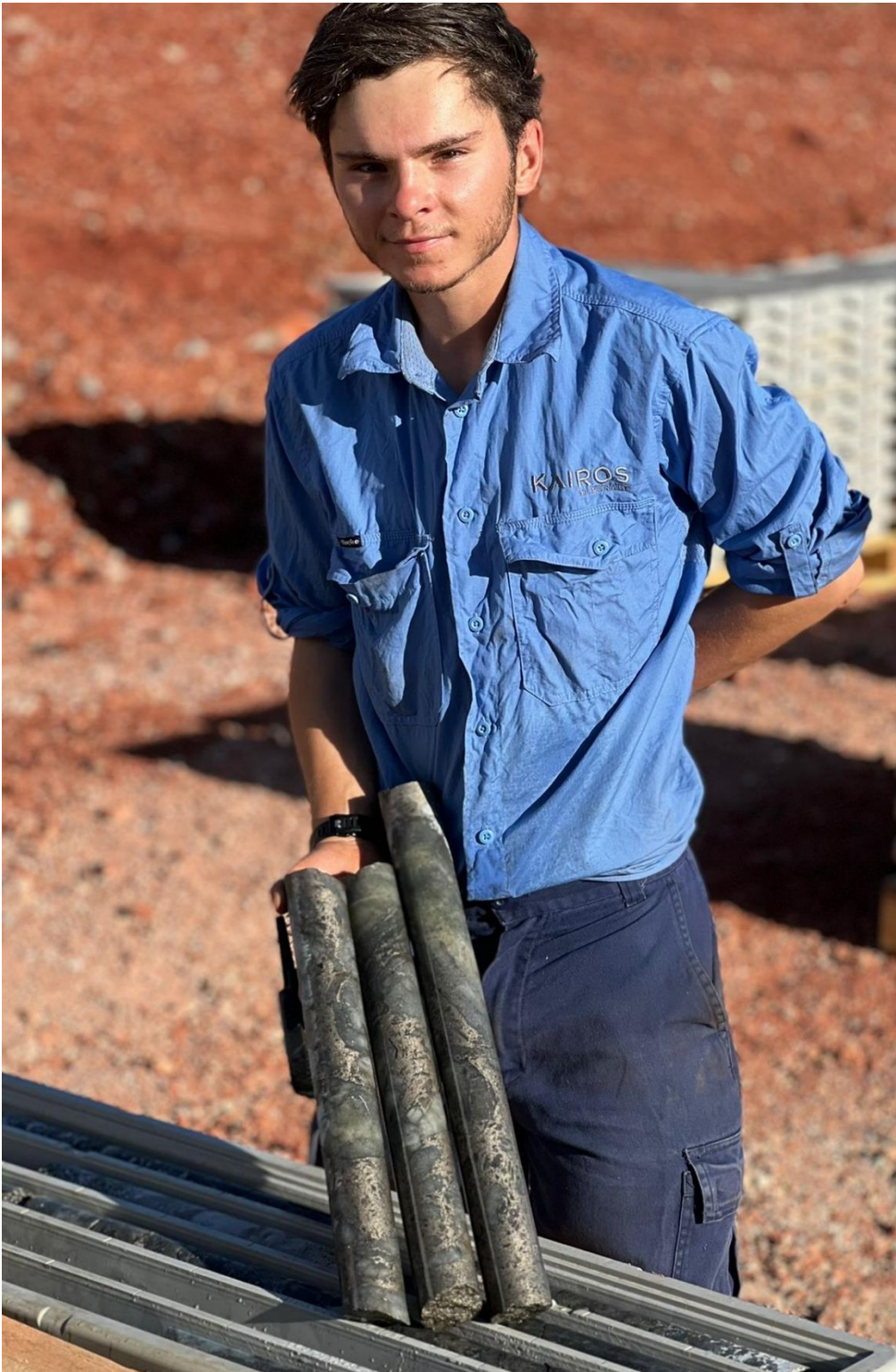
Figure 4. Kairos geologist Will Coussens with core from hole KMYD071 showing extremely silicified and sulphidised (pyrrhotite, pyrite, arsenopyrite) wall rocks at the hangingwall contact of a well mineralised banded iron formation. The mineralisation is typical of the hangingwall sequence and is 15.4m in down-hole thickness at this location at Main Hill prospect (see Figure 5 ).
