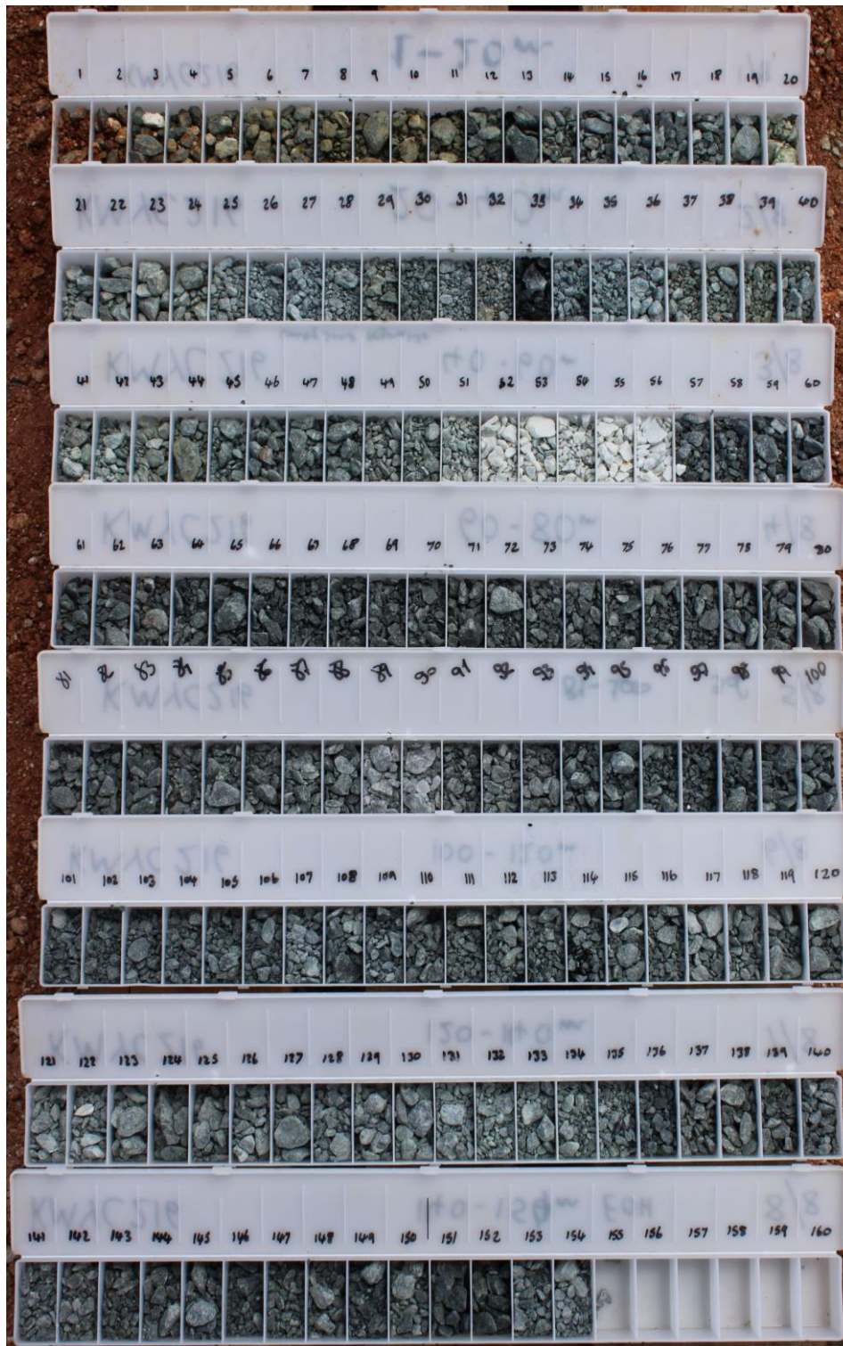
Figure 3. RC chips for hole KMYC216 drilled directly underneath Lucky Sump where surface spodumene-bearing pegmatite samples returned up to 1.91% \text{Li}_2\text{O} . Note the white chips in metres 52-56m. Results pending.
