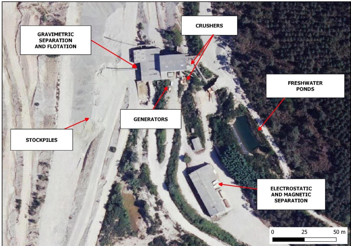
Figure 2. Aerial view of main facilities at San Finx site.
